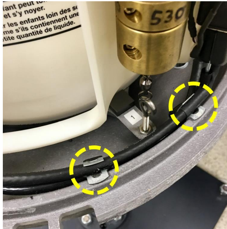
Figure 31. Ensure Internal Wires Secure to the Sides with existing Metal Clamps.
