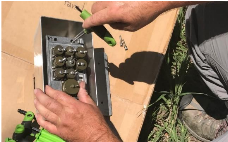
Figure 37. Remove Grape from Grape Shields.
