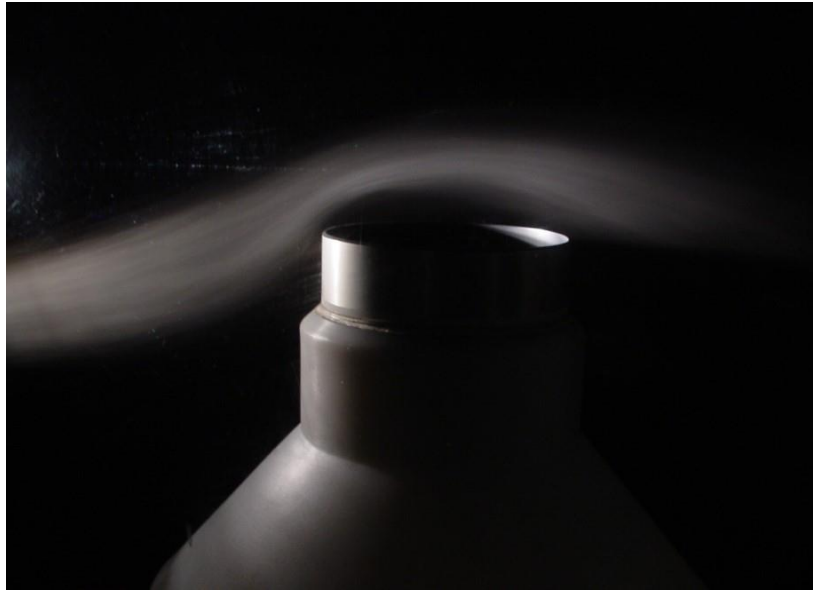
Figure 1. Visual example of wind updrafts at the Primary Precipitation gauge orifice. (Rasmussen et al. 2011).
