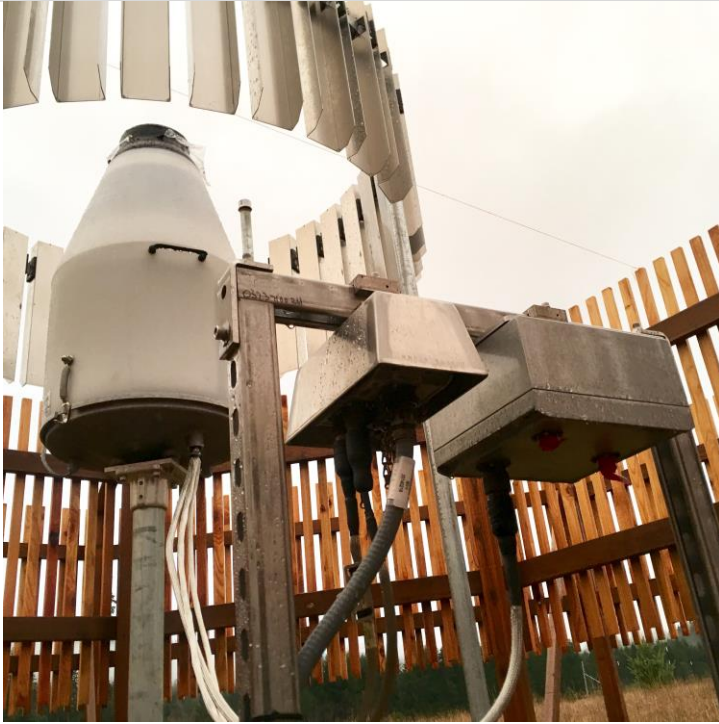
Figure 11. View of the associated Primary Precipitation Gauge Grapes.
