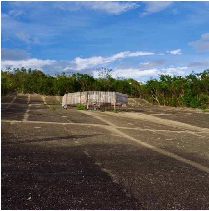
Figure 7. A NEON DFIR within a water catchment basin.
