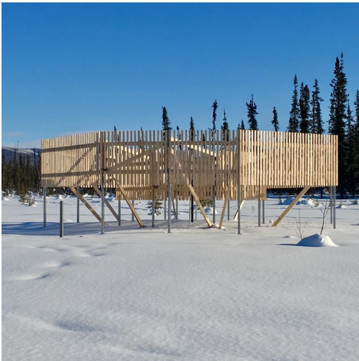
Figure 4. Side view of a NEON DFIR in the winter.
