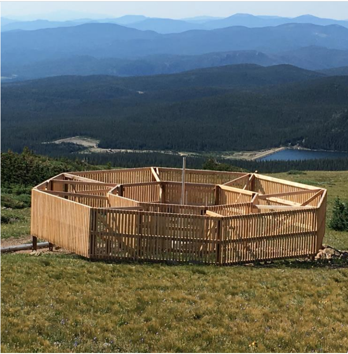
Figure 5. View of the concentric octagonal fences of a NEON DFIR.
