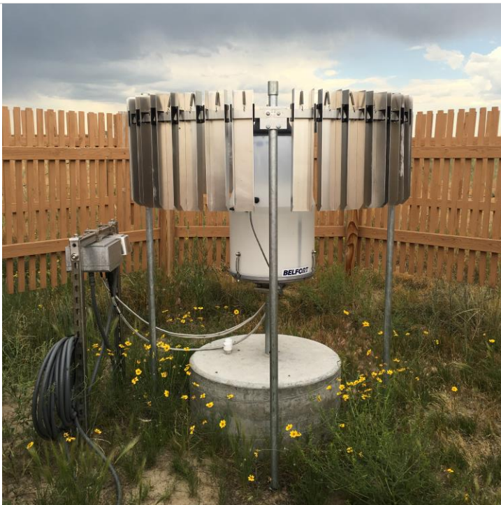
Figure 10. View of the metal Alter shield residing within the two outer concentric octagonal fences. The Primary Precipitation Gauge is inside the Alter shield.
