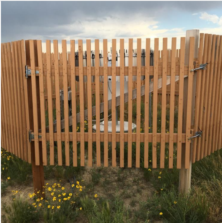
Figure 9. View of the inner DFIR fence and inner fence gate. This also provides an abstract view of the Alter shield and rain gauge.
