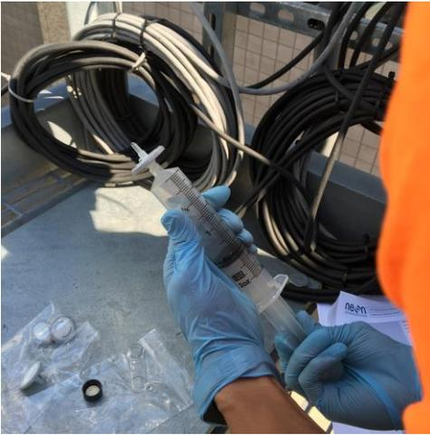
**Step 9.** Tip the syringe up and push on the plunger to squeeze out excess air.
