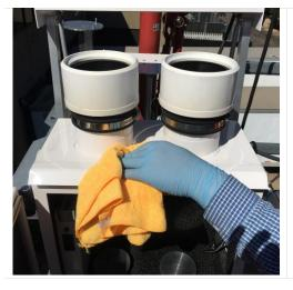
**Step 5.** Clean the top surface of the body of the collector, and wipe down the sides, as well. Re-apply cleaner to the lint-free cloth, if necessary.
