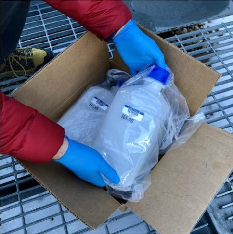
**Step 16.** Place the bagged sample bottle inside the shipping box.
