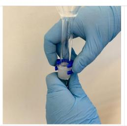
**Step 14.** Carefully remove the Keck clip from the assembled sample train and set aside.
