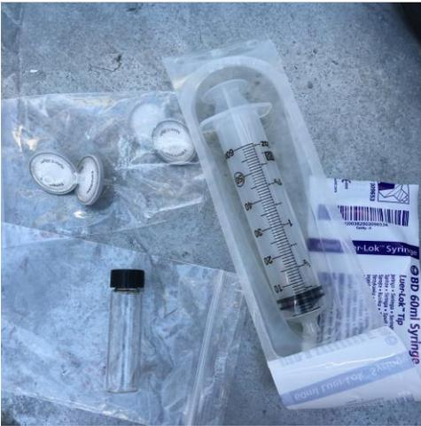
**Step 1.** Locate and stage the 16 mL glass sample vial, 60 mL syringe, and a couple of the 0.2 µm filters in a clean
