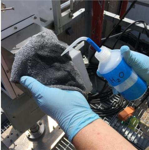
**Step 11.** Spray/squeeze distilled/deionized water onto the lint-free cloth.
