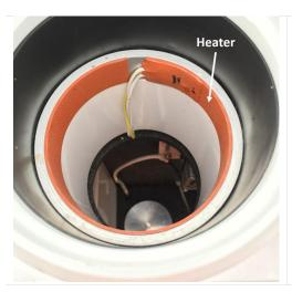
**Step 1.** Check the condition of the strip heaters within each chimney stack. Look for whether the heaters are pulling away from the inside of the chimney.
