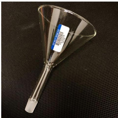
**Step 16.** Locate the lab-provided barcode on the funnel, and scan with your mobile recording app, or record the number on the datasheet.
