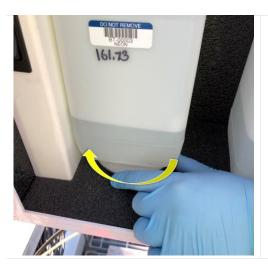
**Step8.** Lower the plastic sample bottle by rotating the metal bottle holder tray **clockwise** until the bottom of the bulb of the thistle tube clears the opening of the sample bottle.
