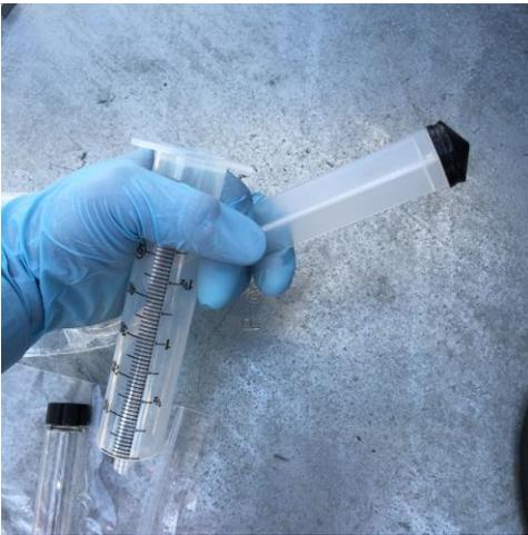
**Step 3.** Remove the 60 mL syringe from its packaging and pull the plunger out by pulling firmly. Hold the syringe plunger in the same hand as the syringe.
