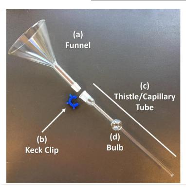
Figure 12. Expanded view of the glass sample train.
