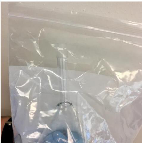
**Step 4.** While still inside the plastic bag, orient the narrow end of the funnel so it is facing towards the resealable bag opening.
