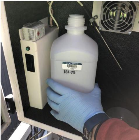
**Step 3.** Remove a clean plastic sample bottle from its plastic bag and place it on the bottle holder.
