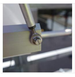
**Step 7.** Inspect the four spherical ball joints at the end of the rear Moving Cover arms. There should be some movement when the arms are slightly twisted (previous Step).
