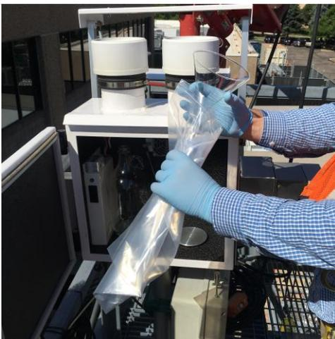
**Step 10.** Carefully hold the glass sample train by the funnel and remove the bottom plastic bag.
