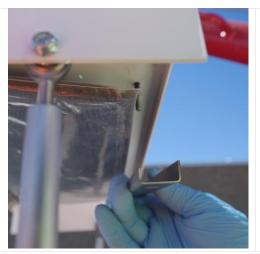
**Step 8.** Press the lid seal towards the other side and hold in place with the aluminum bar from **Step 4** above.
