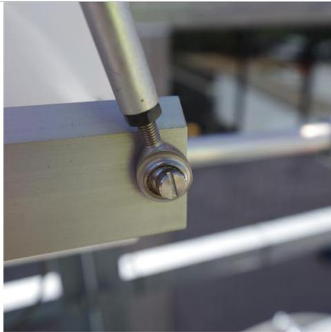
**Step 7.** Inspect the four spherical ball joints at the end of the rear Moving Cover arms. There should be some movement when the arms are slightly twisted (previous Step).
