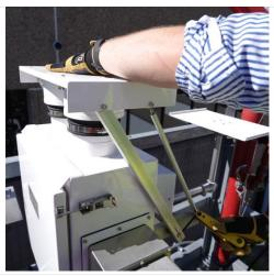
**Step 5.** Hold the lid firmly on top of the chimneys and retighten the cap screws firmly to secure the drive arms.
