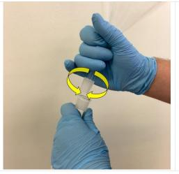
**Step 15.** With a slight twisting motion, carefully disassemble the funnel from the thistle tube.
