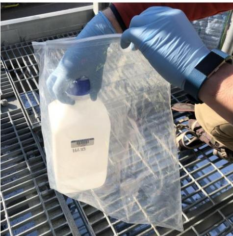
**Step 15.** Place the empty isotope analysis sample bottle back into a 16 X 16", 4 mil, resealable plastic zip bag and seal.
