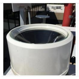
**Step 15.** Ensure the top of the funnel is below the top of the chimney sides as displayed in the corresponding photo.
