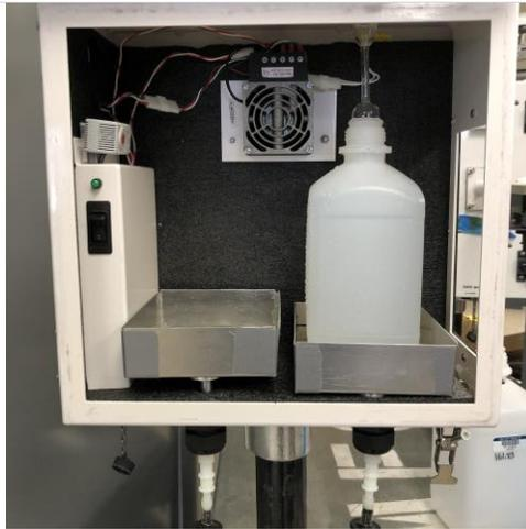
**Step 4.** If using overflow catch basins, and evidence of overflow on the sample bottles exist, ensure the overflow basin drained properly. Note condition in the fulcrum application.
