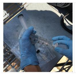
**Step 4.** Attach the 0.2  $\mu$ m filter and secure to the Luer-Lok tip at the end of the syringe. Continue holding the syringe plunger in the same hand.
