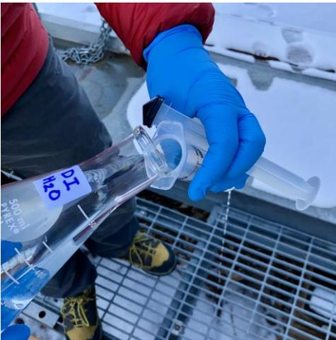
**Step 17.** Rinse the syringe and plunger with deionized (DI) water three times, and let dry completely for the next collection.
