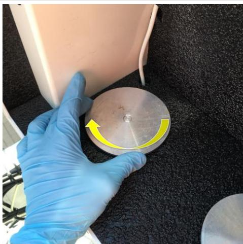
**Step 2.** Lower the sample bottle holder by turning it clockwise until it is all the way down.
