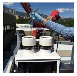
**Step 11.** Gently place the sample train into the same chimney that the sample bottle is under.
