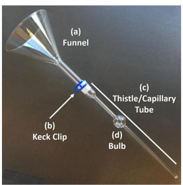
Figure 11. A fully assembled glass sample train includes:
