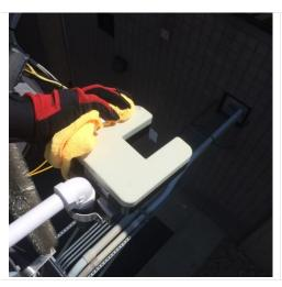
**Step 8.** Clean the Precipitation Sensor. Top, sides, bottom, as well as within the "U" shaped part of the sensor.
