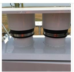
**Step 3.** Observe the Moving Cover as it closes. Again, the movement should be smooth and consistent.
