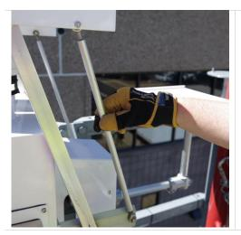
**Step 6.** Inspect the arms of the moving cover. Gently twist the rear arms, they should move slightly and should not be seized.
