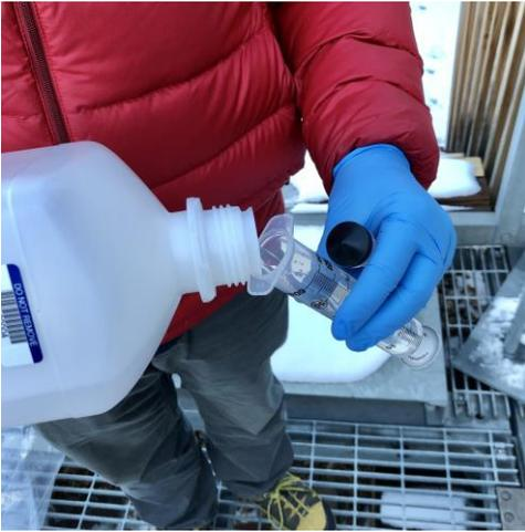
**Step 5.** *If* the sample volume in the isotope sample bottle is greater than 30 mL **and** a used syringe is being used, rinse the syringe with sample water from the isotope sample bottle at least once and up to three times with sample. To rinse syringe, pour in water, cap with plunger and shake for 15 seconds. After rinsing syringe push sample water through filter to saturate the filter.
