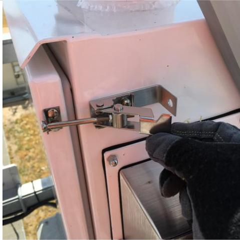
**Step 1.** Unlatch the two latches holding the closed door and open the door.
