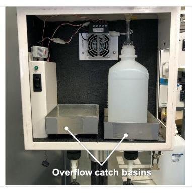
Figure 6. Overflow catch basins placement.
