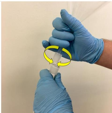
**Step 15.** With a slight twisting motion, carefully disassemble the funnel from the thistle tube.
