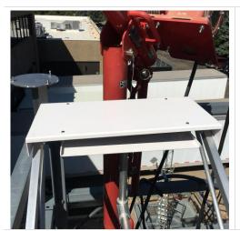
**Step 2.** As the Moving Cover opens, observe its full range of motion. Movement should be smooth and consistent.
