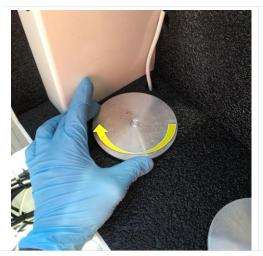
Step 2. Lower the sample bottle holder by turning it clockwise until it is all the way down.
