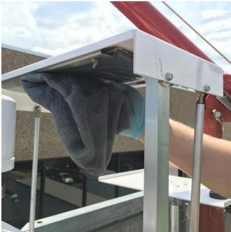
**Step 12.** Clean the underside of the seal on the Moving Cover with the distilled/deionized water.
