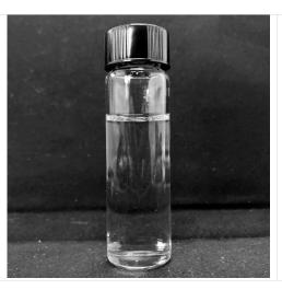
**Step 11.** Fill the bottle so it is  $^{80}$ % full ( $^{20}$ % headspace). This is 12-13 mL of sample.
