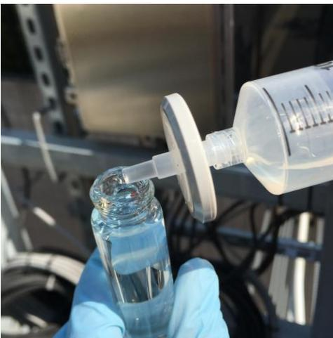
**Step 10.** Apply even pressure plunging the sample through the filter into the glass vial.
