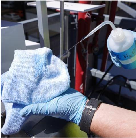
**Step 10.** Spray or squeeze distilled or DI water onto the lint-free cloth.
