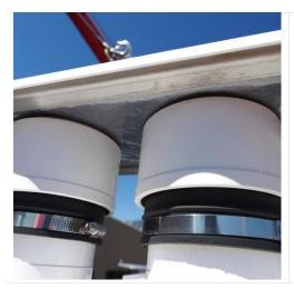
**Step 6.** Repeat opening and closing the Moving Cover to ensure that the lid seals properly on the chimneys.
