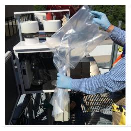
**Step 9.** Hold the assembled sample train so the funnel is up and remove the plastic bag that is over the funnel only.
