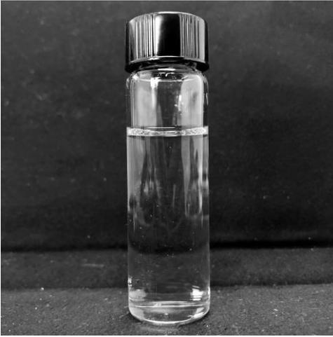
**Step 11.** Fill the bottle so it is ~80% full<sup>1</sup> (~20% headspace). This is 12-13 mL of sample.
