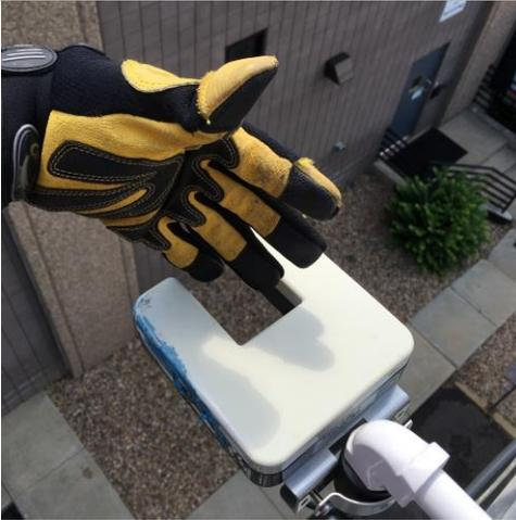
**Step 1.** Wave fingers or hand slowly vertically in-and-out of the Precipitation Detector until the Moving Cover begins to open.
