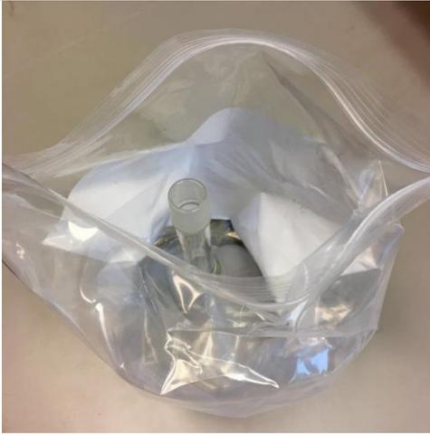
**Step 5.** Place the funnel with the wide end at the bottom on a stable surface, and open the plastic bag, but do not remove the funnel just yet.
