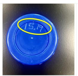
**Step** 31. Record the tare weight etched on the cap.
