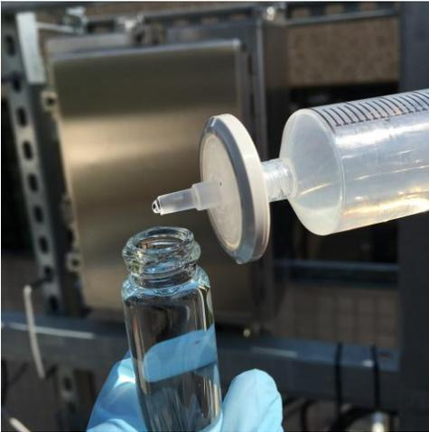
**Step 6.** Rinse sample vial with filtered water by adding a small portion to the vial, capping and shaking. Repeat three times.
