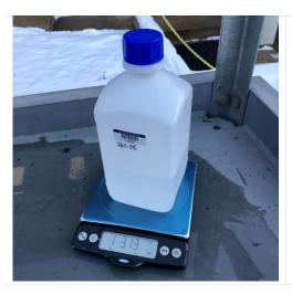
Step 29. Place the capped sample bottle on the scale and record the weight (in grams to the hundredths place).
