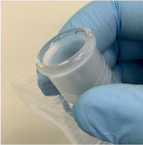
**Step 6.** Open the plastic bag holding the thistle tube and have the frosted glass end pulled out. Keep rest of thistle tube within the bag.
