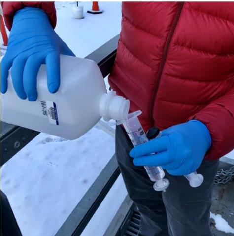
**Step 7.** Fill the syringe to the 30 mL mark. If there is not enough of the collected sample to fill to the 30 mL mark, pour in the entire sample.
