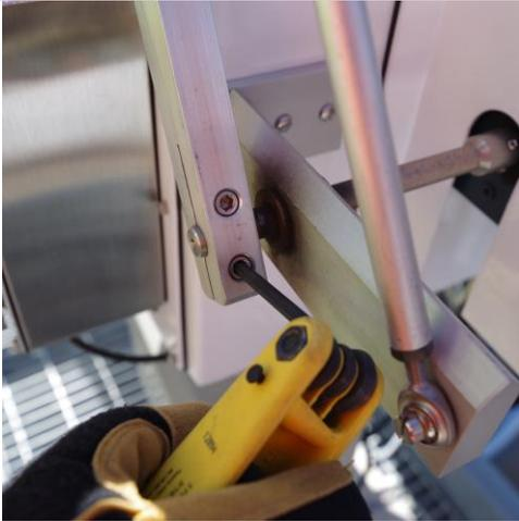
**Step 4.** Loosen the 4 cap screws holding the drive arms to the motor axles so the lid comes down on top of the chimneys.
