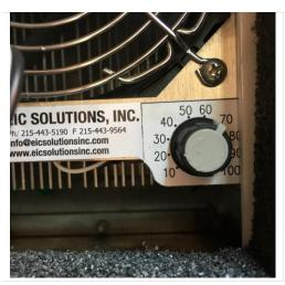
**Step 2.** Verify the set point is ~77 °F on the Temperature Controller on the Thermo-electric chiller (see **Figure 5** and **Figure 10**).
