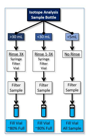
Figure 14. Flow Diagram for Isotope Sub-Sampling.
