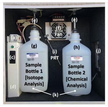
**Figure 5.** The inside view of the environmental enclosure.
