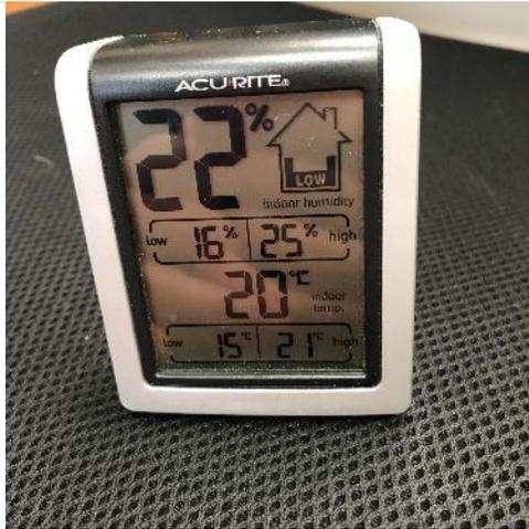
**Step 4.** Record the temperature showing on the indoor thermometer placed within the enclosure.
