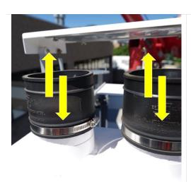
**Step 5.** Once the hose clamp is loosened, pull up on the gasket to raise, or push down on the gasket to lower.
