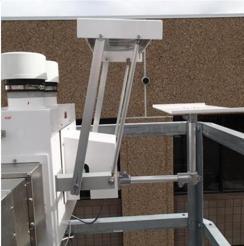
**Step 2.** Allow the Moving Cover to open until it is about half-way to fully open, or until the lid is vertical, and flip the power switch (see **Figure 5**) to the off position.
