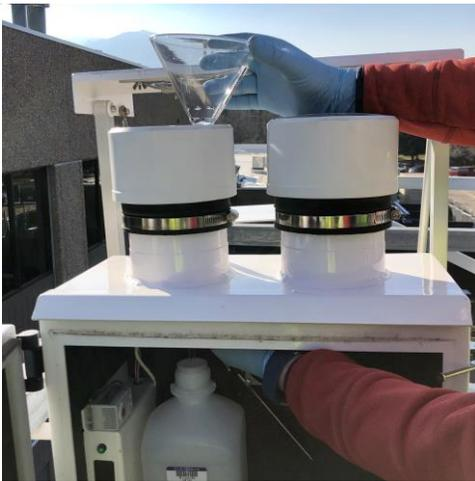
**Step 12.** Guide the thistle tube into the sample bottle and help settle the funnel into the chimney.
