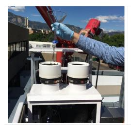
**Step 11.** Gently place the sample train into the same chimney that the sample bottle is under.
