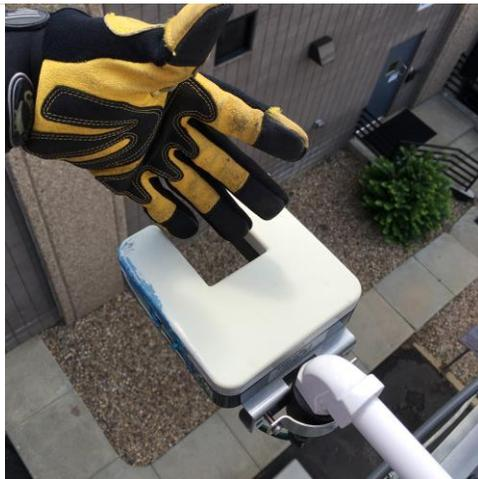
**Step 5.** Slowly wave a hand (with fingers spread open) vertically in-and-out of the Precipitation Detector until the Moving Cover begins to open.
