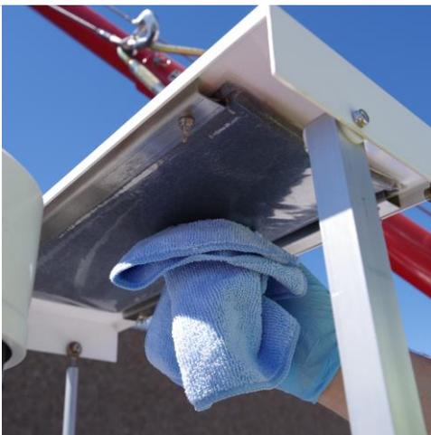
**Step 11.** Clean the underside of the lid seal with the distilled/deionized water, or ethanol in cold weather.
