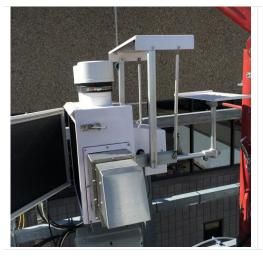
**Step** 6. Allow the Moving Cover to open until it is about halfway to fully open, or until the funnels are fully uncovered, and flip the power switch (see **Figure 5**) to the off position.
