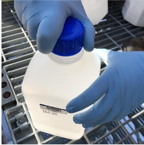
**Step 13.** Tighten the cap on to the sample bottle.
