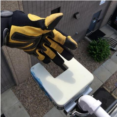
**Step 1.** Slowly wave a hand (with fingers spread open) vertically in-and-out of the Precipitation Detector until the Moving Cover begins to open.
