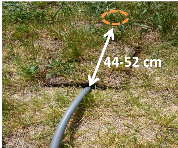
Figure 4. The Soil Heat Flux sensor is located approximately 44-52 cm (~17-20 inches) in front of the location where the cable enters the soil (dashed orange circle).
