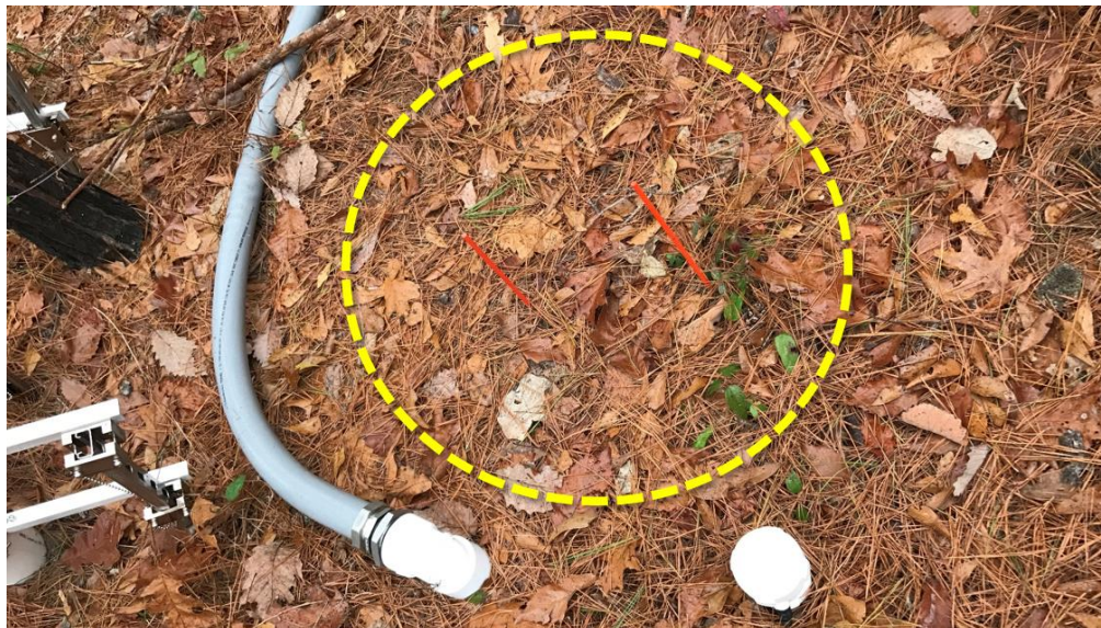
Figure 5. Fiberglass Snow Stakes Identifying the Soil Heat Flux location in a Soil Plot (SP) (Domain 08, Talladega National Forest TIS Site).
