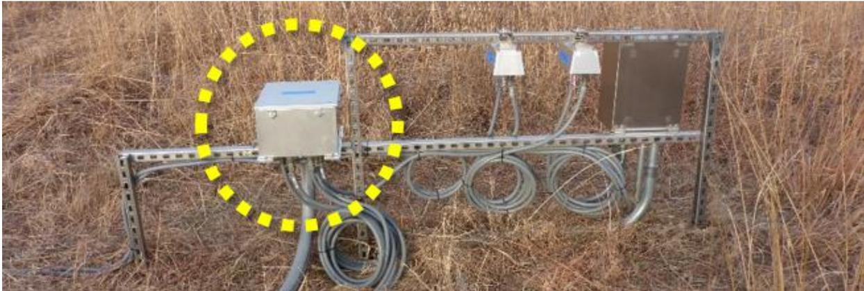
Figure 14. Grape Box/Enclosure on Arbor for Soil Temp & CO<sub>2</sub> Sensors (D06 KONZ).
