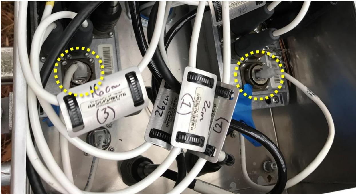
Figure 15. Disconnect the RJF/Eth to Comm Connection.
