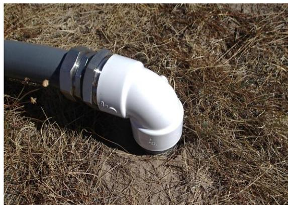
**Figure 8.** Top of Soil Temperature Profile Assembly.
