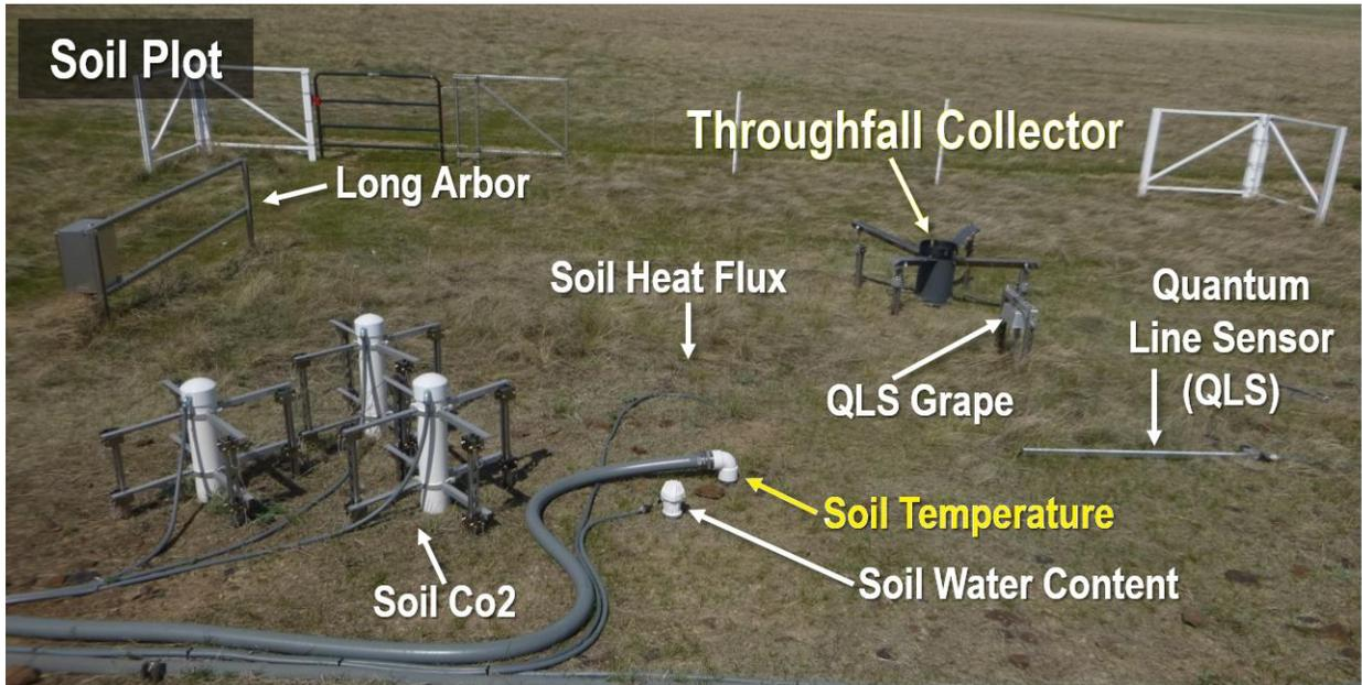
**Figure 6.** Soil Plot 1 (Domain 10, CPER) with Cattle Fencing (Not Shown: Device Post, Short Arbor, HMP, Apogee, and NR01).
