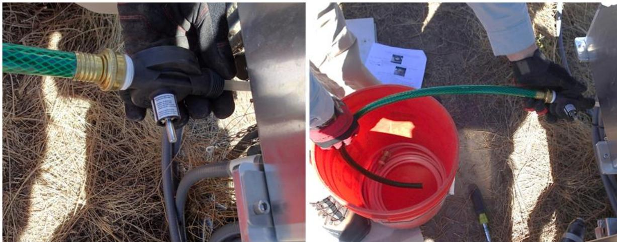
Figure 11. Close-up and expanded view of drill pump connection to sensor drainage tube and garden hose.
