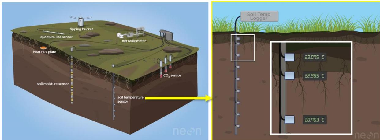
**Figure 1.** Soil Temperature 4-Wire PRT Sensors Vertical Profile in a Soil Plot.
