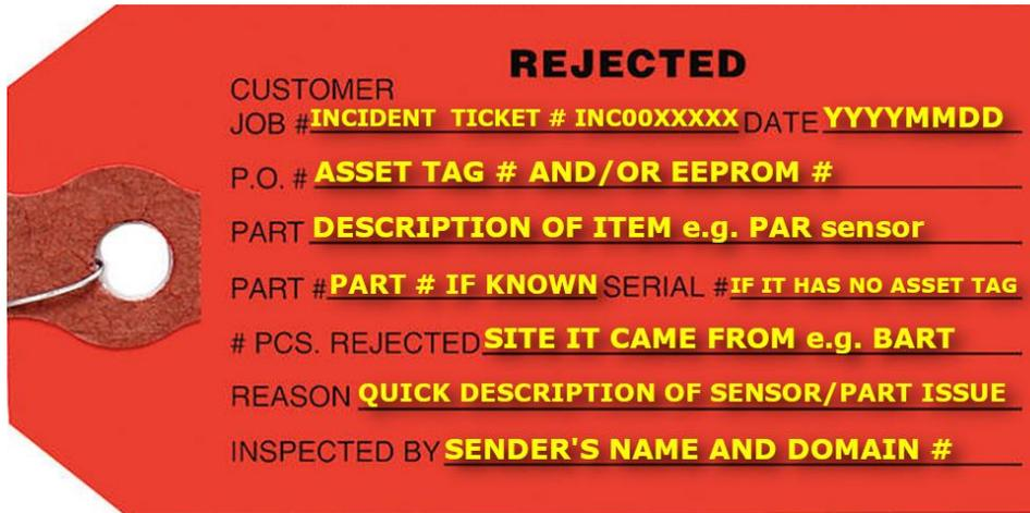
**Figure 16.** Red Rejected Tag for Defective Assets.
