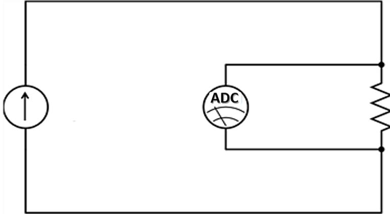
Figure 5. Four-wire Measurement for a PRT.
