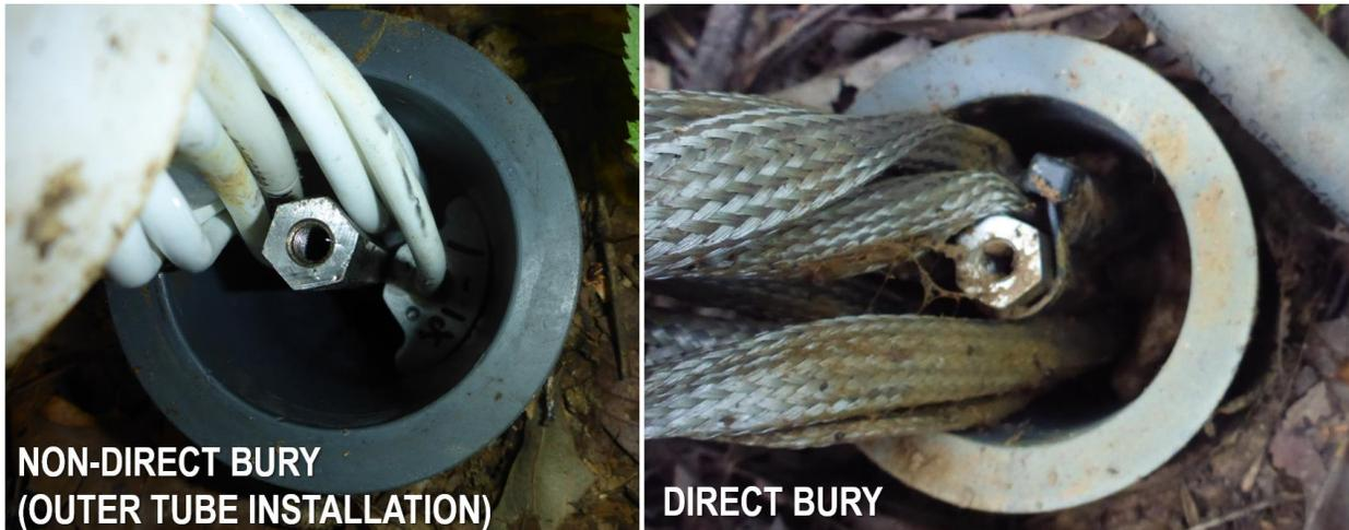
Figure 2. Non-Direct Bury (Outer Tube Installation) and Direct Bury Sensor Installations.
