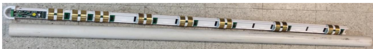
Figure 1. Soil Water Content and Salinity Profile Instrument with PVC Outer Tube (Below Instrument).
