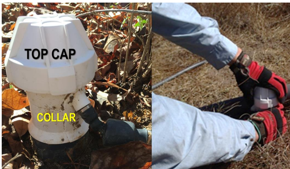
Figure 8. Brace Collar (right hand in picture on right) when Removing the Top Cap to Prevent Assembly Movement.
