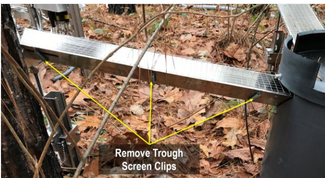
Figure 14. Remove Screen Clips to Remove Screen from Troughs.
