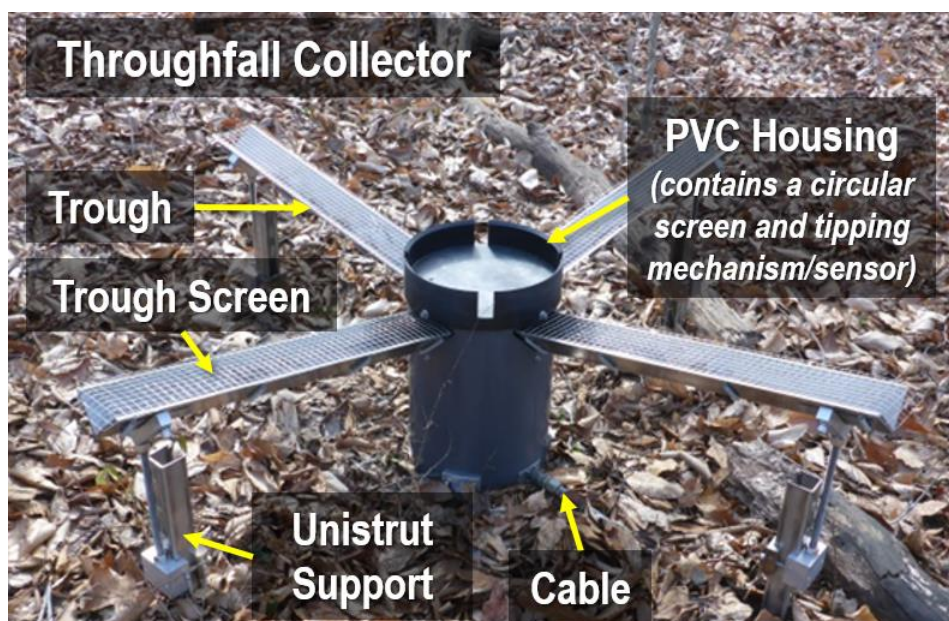
Figure 1. Throughfall Exterior Components.
