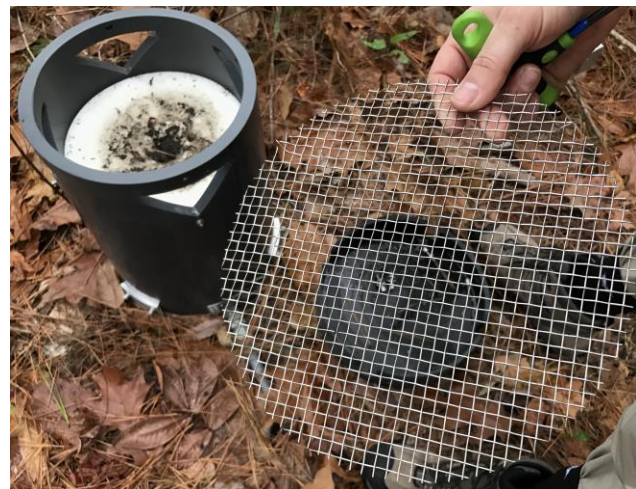
Figure 7. Remove Screens to Clean Collector.
