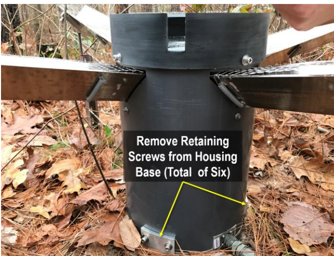
Figure 15. Remove Collector Body from Sensor Base.
