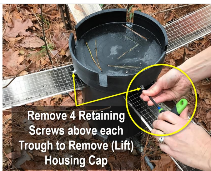
Figure 11. Remove Housing Cap.
