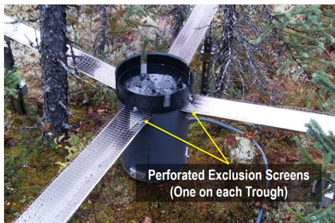
Figure 12. Remove Four Perforated Exclusion Screens.
