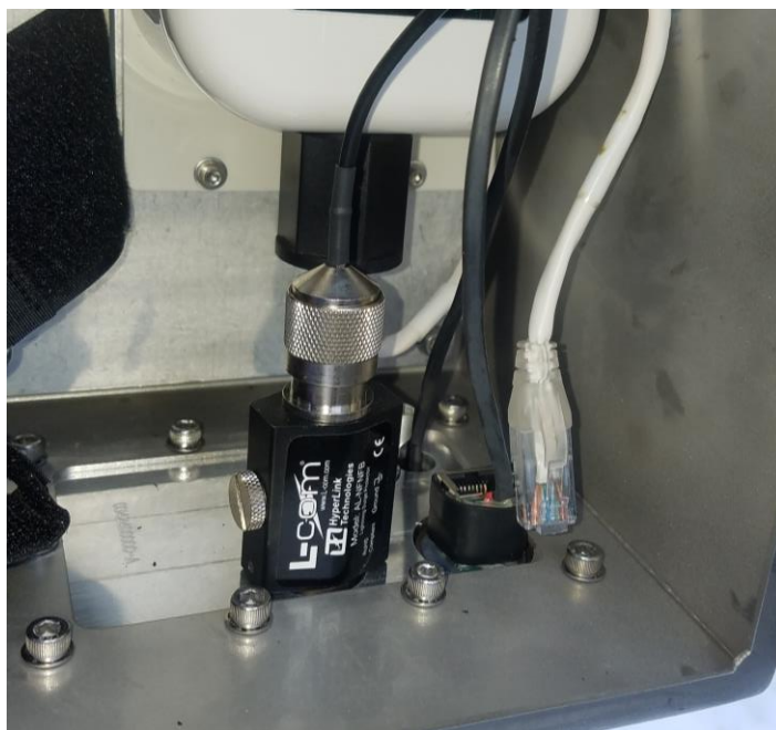
Figure 27. Disconnect Radio Connector (Bottom Right Corner of Combo Box, D18 TOOK)
