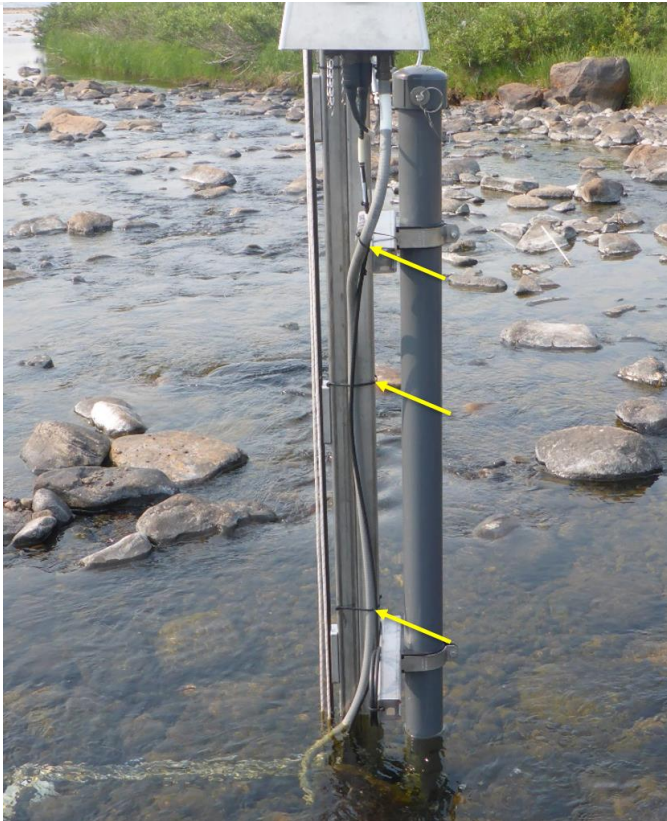
Figure 18. Secure Cables using Zip Ties
