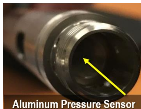
Figure 6. Sensitive Pressure Sensor Diaphragm (Level TROLL 500 without Nose Cone) ER[03]
