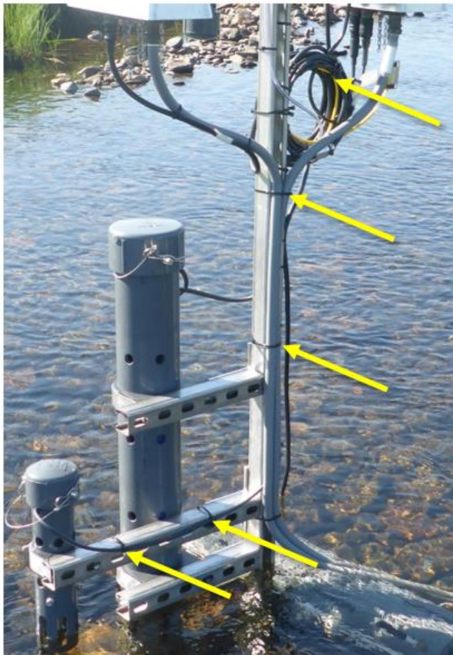
Figure 23. Secure Cables using Zip Ties (D18 OKSR)
