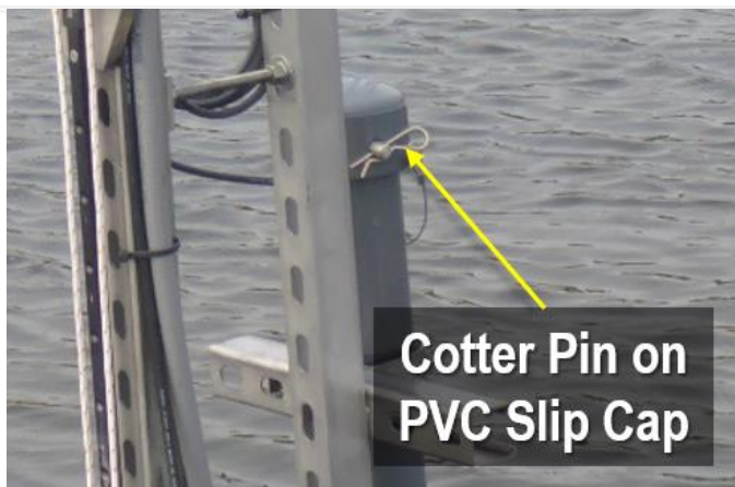
Figure 14. Remove Cotter Pin from PVC Slip Cap to Access Sensor
