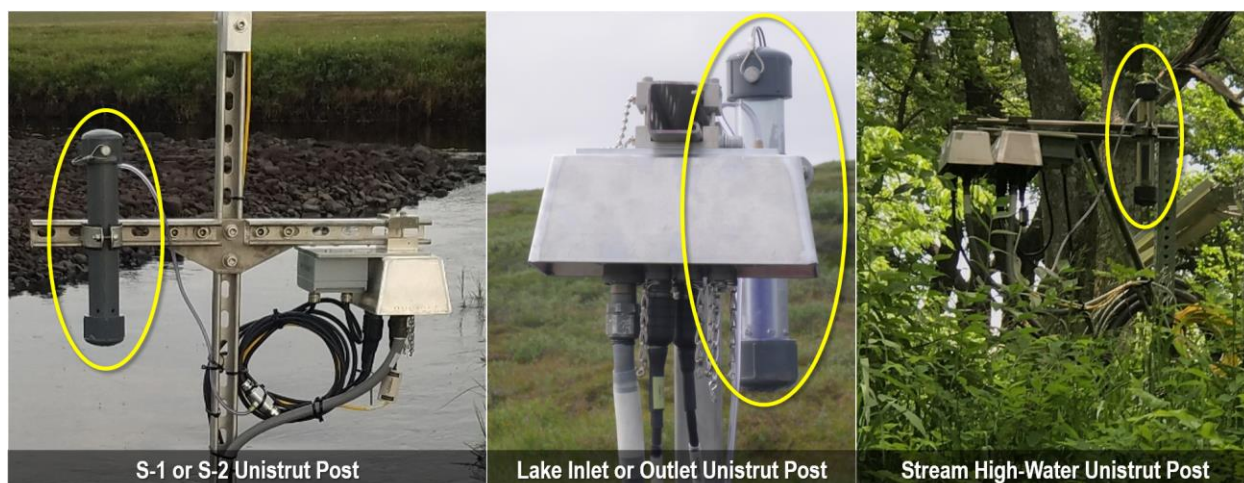
Figure 7. Level TROLL 500 Desiccant Canister Locations (Left to Right: D18 TOOK, D09 PRLA, D06 KING)
