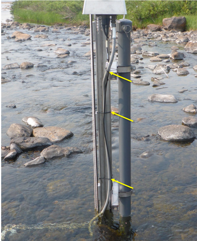
Figure 18. Secure Cables using Zip Ties
