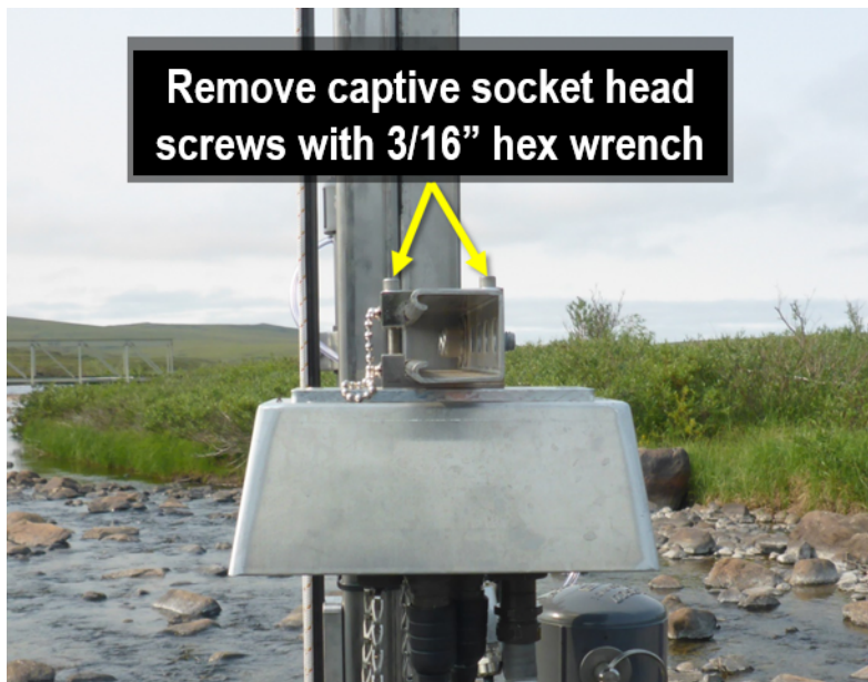
Figure 11. Remove Grape Shield with 3/16" Hex Wrench
