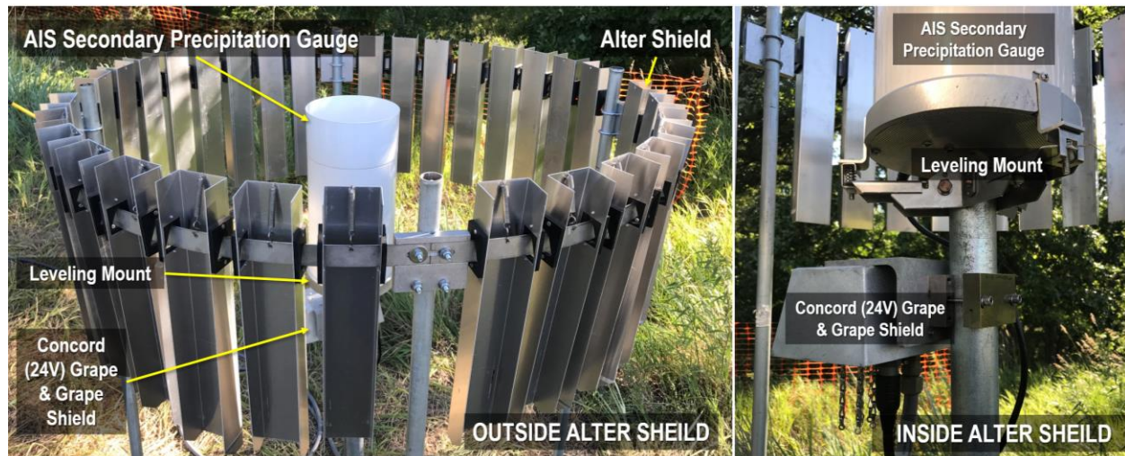
Figure 3. AIS Secondary Precipitation Gauge with Alter Shield at Aquatic Sites
