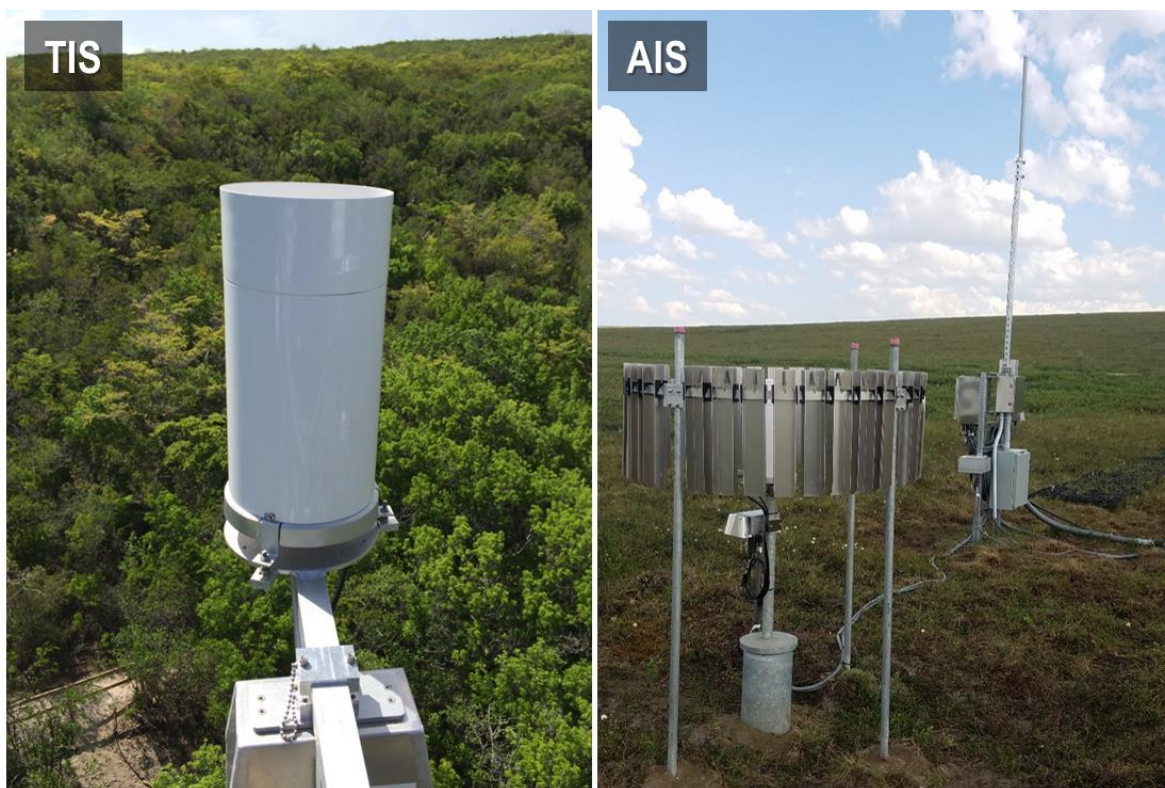
Figure 4. Secondary Precipitation Gauge: TIS Site (Left) Domain 04, GUAN, AIS Site (Right) Domain 18, TOOK.
