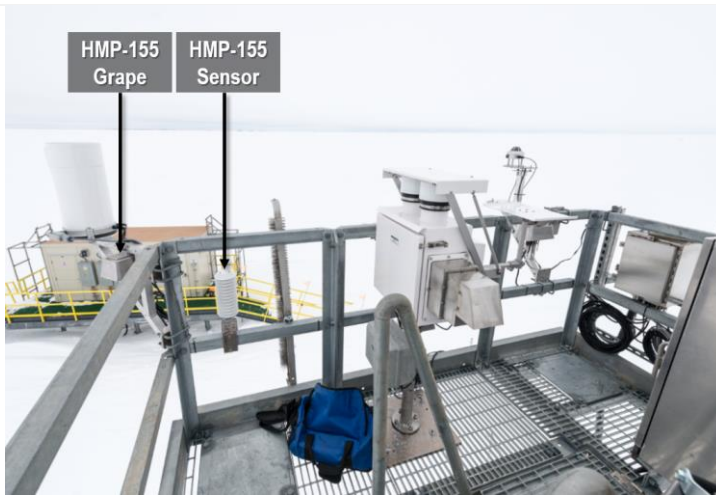
Figure 13. Humidity & Temp Sensor & Subsystem TIS Tower (D18 BARR).
