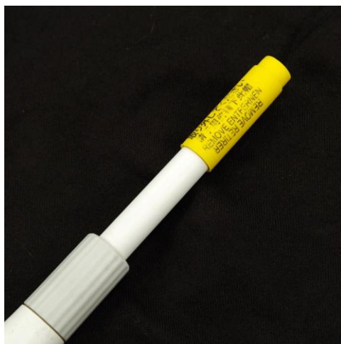
Figure 12. Sensor protective cover over the PTFE Filter during handling, cleaning, and transport.
