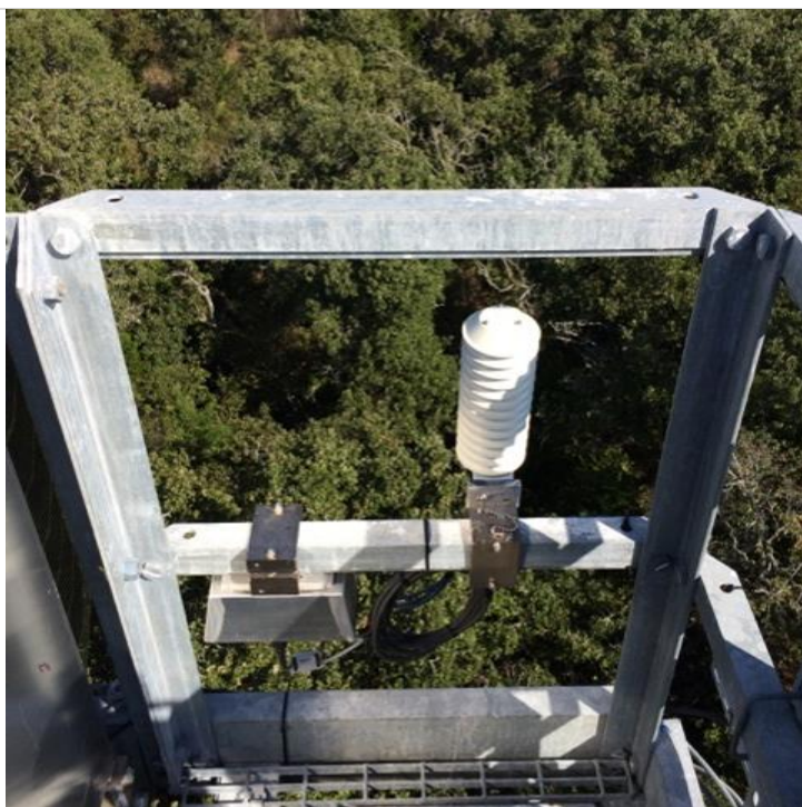
Figure 8. TIS Tower mounted Humidity and Temperature Sensor with associated Grape.
