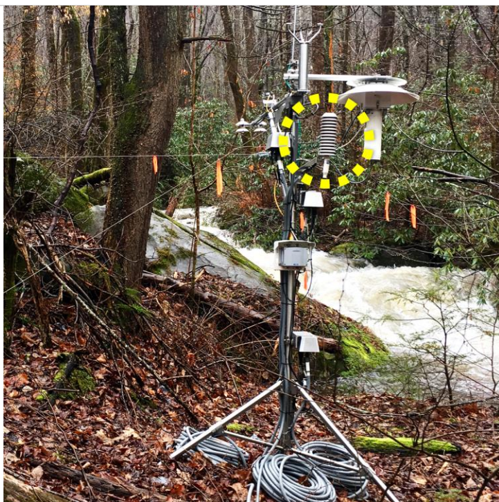
Figure 10. Humidity and Temperature Sensor mounted on an AIS Met Station.
