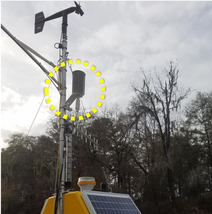
Figure 11. Humidity and Temperature Sensor on the Met Mast of an AIS Buoy.
