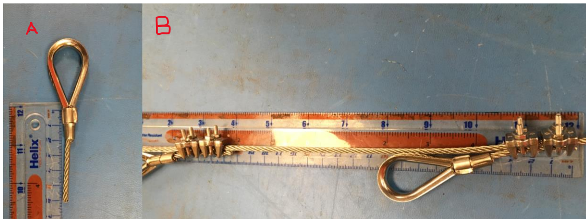
Figure 2. (A) image of a single side connector. (B) Two side connectors attached to a main line.
