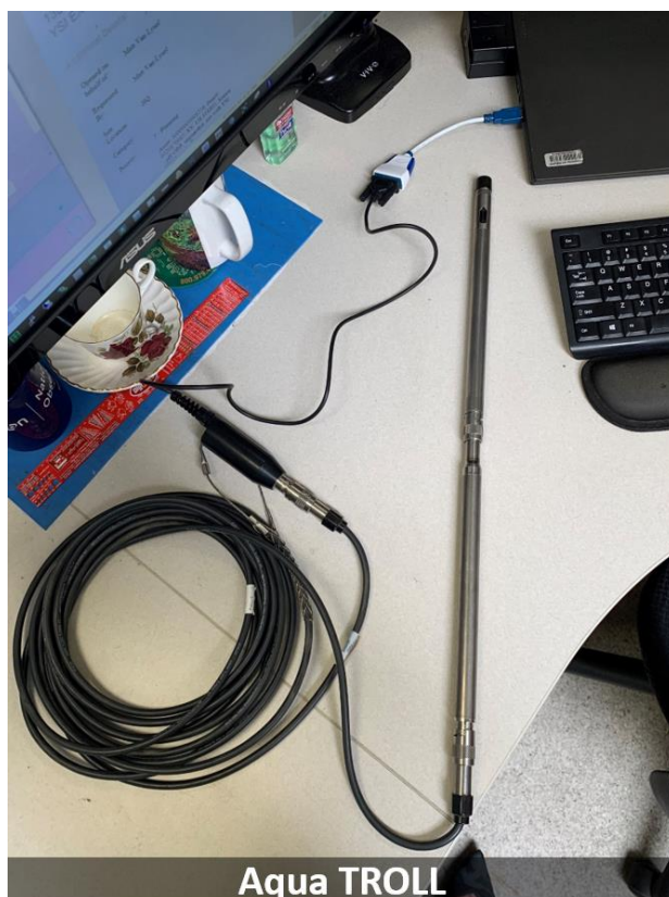
Figure 1. Aqua and Level TROLL Connecting to a Laptop
