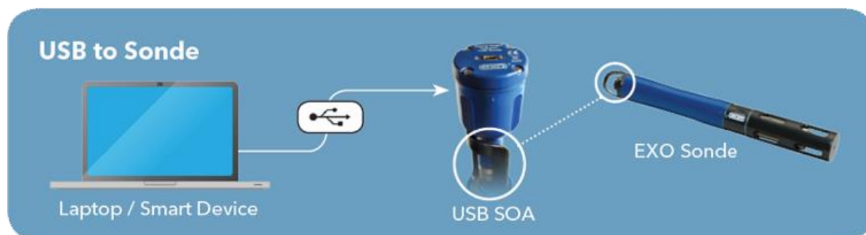
Figure 1. USB to Sonde Connection Method
