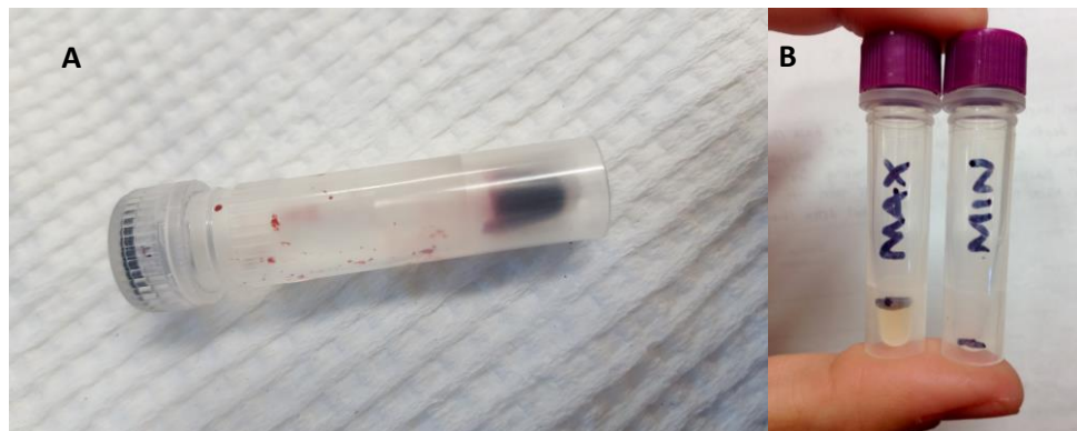
Figure 5. (A) Ideal volume of blood sample (50 microliters). (B) Minimum (20 microliters) and maximum sample volumes (50 microliters) needed for serological analysis.
