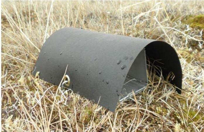
Figure 17. Folding Sherman trap (3"x3.5"x9") covered with 12"x12" tar paper cover in Barrow, AK - from Ott 2012. Credit: Kaithryn Ott.
