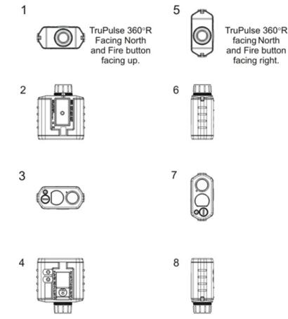
Figure 11. TruPulse 360R Laser Rangefinder compass calibration routine
