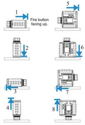
**Figure 9.** TruPulse 360R Laser Rangefinder tiltsensor calibration routine
