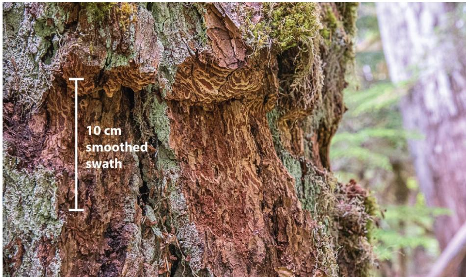
**Figure 22.** Preparation of the bole surface for dendrometer band installation on a deeply fissured Douglas Fir (*Pseudotsuga menziesii*) at the D16 WREF site.
