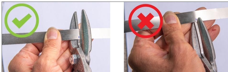
**Figure 4.** (Left) Correct metal-snip technique for cutting the measurement window in a dendrometer band. (Right) Incorrect technique using the tip of the metal snips will result in burrs and band deformation.
