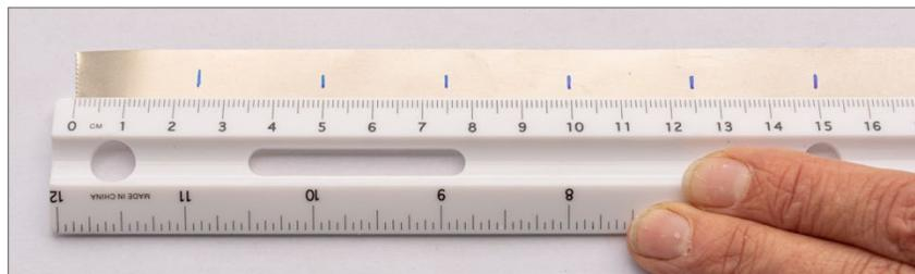
**Figure 3.** Dendrometer band material marked every 2.5 cm for cutting ‘collars’ in preparation for installation in the field.
