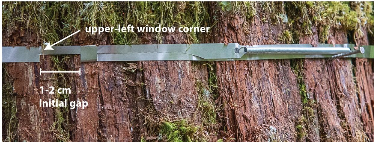
**Figure 24.** Installed dendrometer band with a 1-2 centimeter initial gap in the measurement window. The band is rotated such that the entirety of the measurement window and the spring are fully appressed to a smoothed section of the bole.
