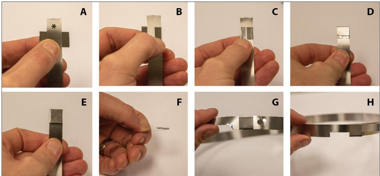
**Figure 23.** Fabricating the dendrometer band buckle with the collar after fitting the band to the tree and cutting to the desired length. The asterisk in **A** denotes the outward-facing side of the band marked in the previous step.
