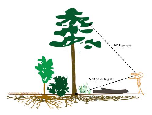
Figure 6 Measuring sample height using a laser rangefinder
