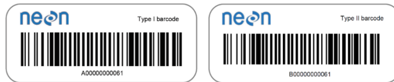
Figure 5. (Left) Example of a Type I barcode. Large-size, field-tolerant, with prefix of 'A' followed by 11 numbers. (Right) Example of a Type II barcode. Large-size, cryo-safe, with prefix of 'B' followed by 11 numbers.
