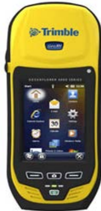
Figure 11. GPS receiver Geo XH 6000
