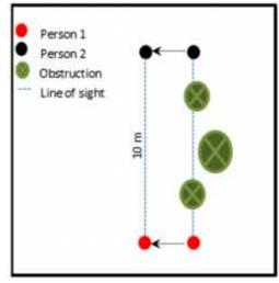
Figure 17. Alternative strategy when obstructions are in line of sight during plot delineation
