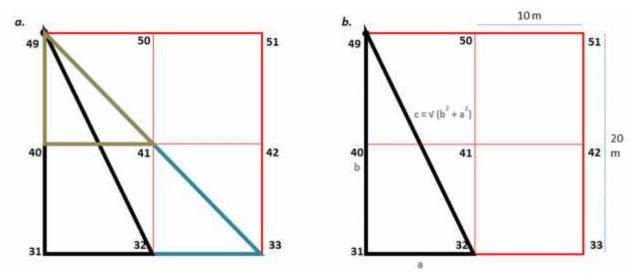
Figure 18. Hypotenuse option to verify plot delineation measurements;
