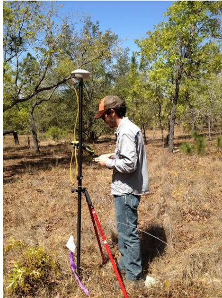
**Figure 8.** GeoXH 6000 set up for high accuracy data collection.
