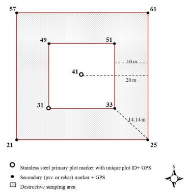
**Figure 7.** Plot layout and marker positions for 40 m by 40m Distributed Base Plots
