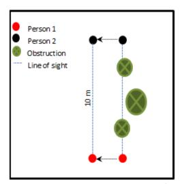
Figure 18. Alternative strategy when obstructions are in line of sight during plot delineation
