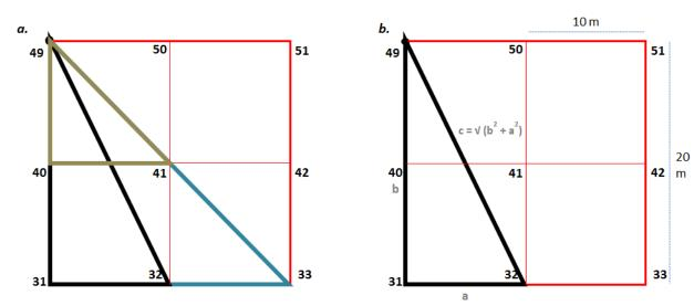
Figure 19. Hypotenuse option to verify plot delineation measurements
