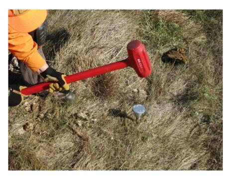
Figure 14. Use a sledgehammer to seat the cap and drive the rod to the desired position
