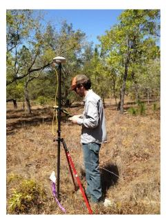
**Figure 8.** GeoXH 6000 set up for high accuracy data collection.
