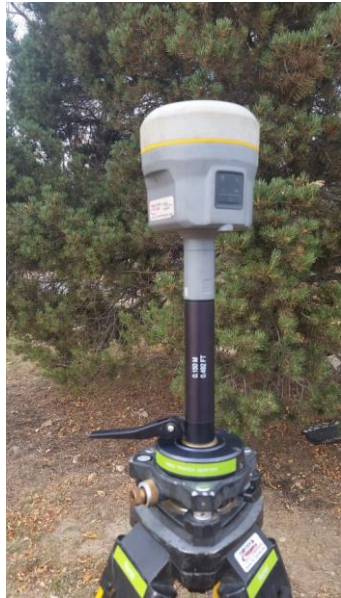
Figure 27. Base station setup.
