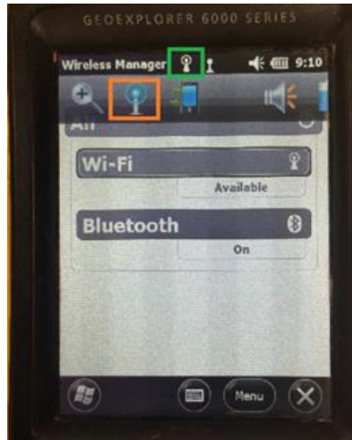
Figure 12. Trimble Wi-Fi symbol setup
