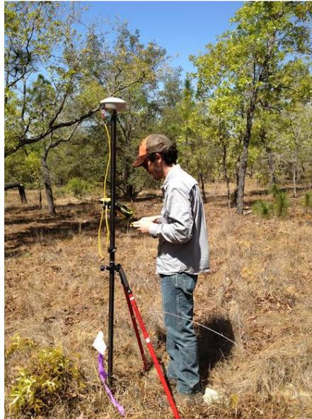
**Figure 14.** GeoXH 6000 set up for high accuracy data collection.
