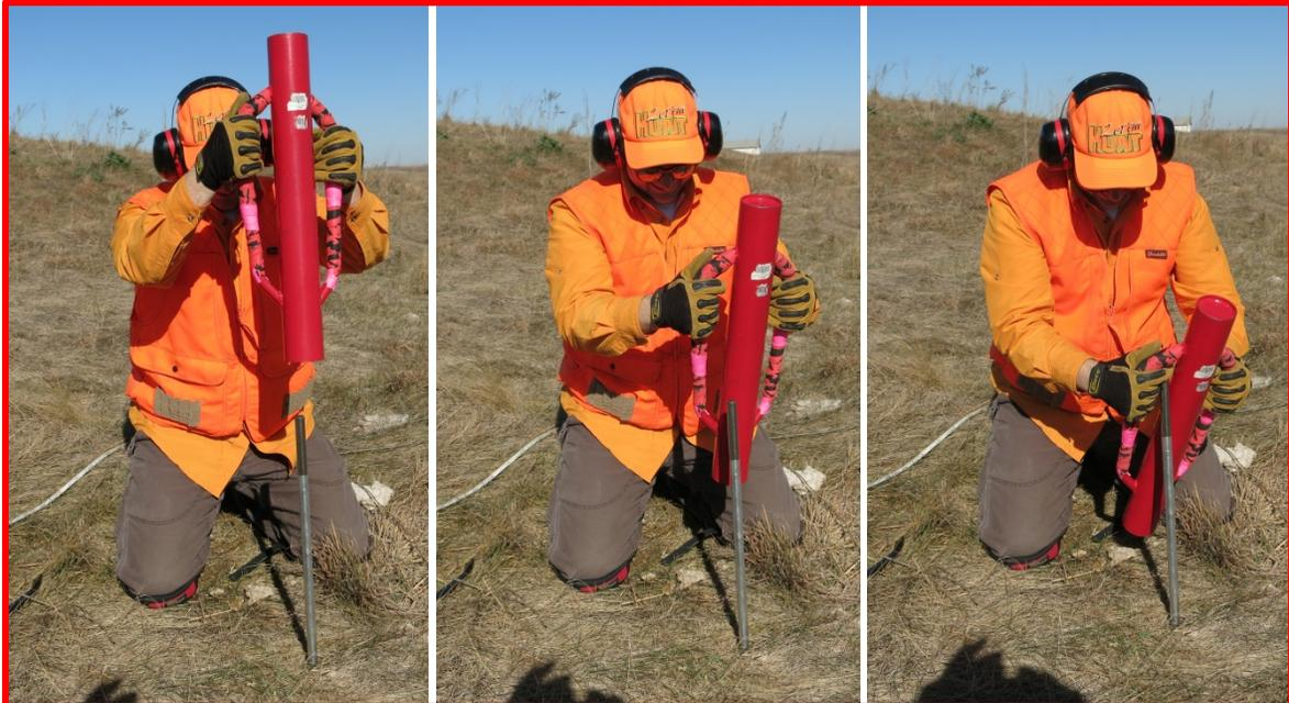
**Figure 29.** Do not lift the post driver above the top of the rod during the striking motion as the worker could injure their leg or hand
