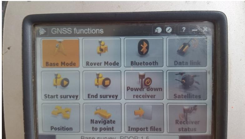
**Figure 39.** Base mode highlighted orange
