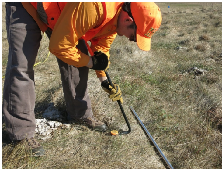
Figure 12. Removing a pre-existing temporary plot marker with a pry bar.
