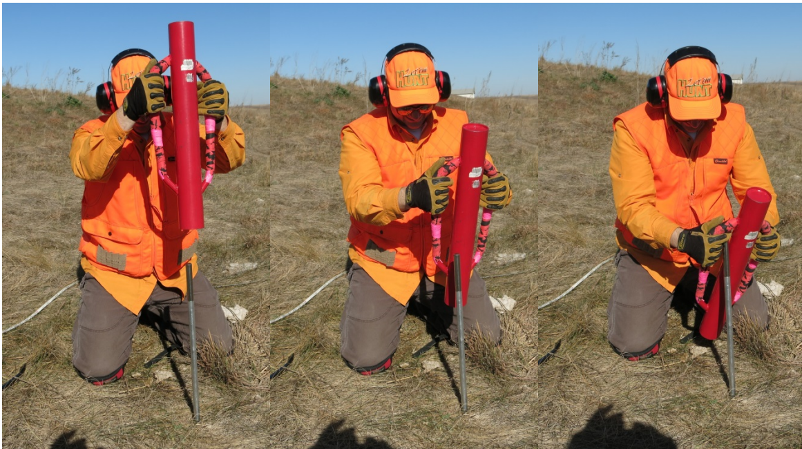
Figure 14. Demonstration of a dangerous method using the post driver. If the post driver is raised above the rod (first picture) during the upward swing it can miss the rod (second picture) and injure the workers hand or leg (third picture).
