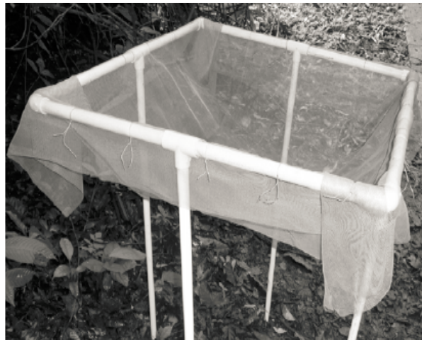
Figure 3. Fully constructed elevated litter trap. NEON traps will have legs attached on corners rather than center (photo from Muller-Landau and Wright 2010).
