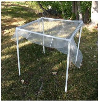
Figure 5. Fully constructed elevated litter trap.
