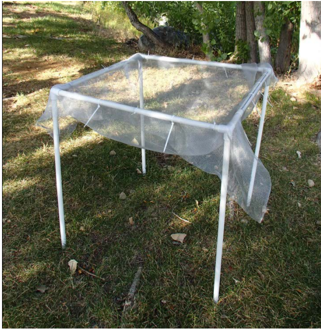
Figure 3. Fully constructed elevated litter trap. .
