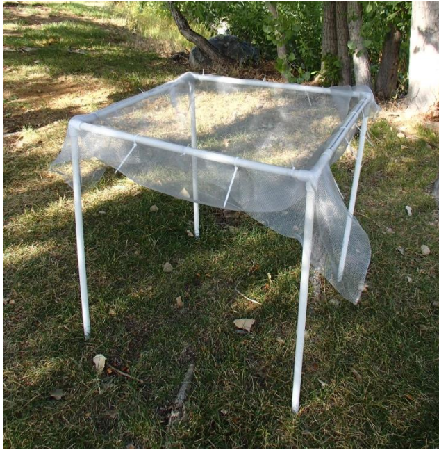
Figure 4. Fully constructed elevated litter trap.
