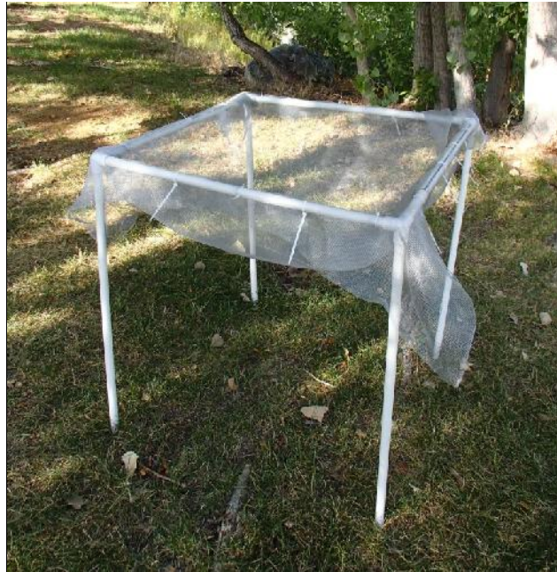
Figure 4. Fully constructed elevated litter trap.
