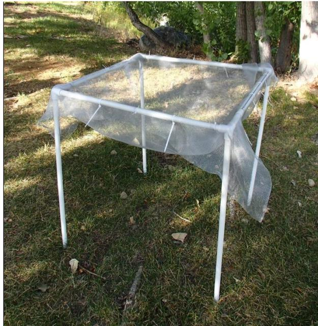
Figure 5. Fully constructed elevated litter trap.
