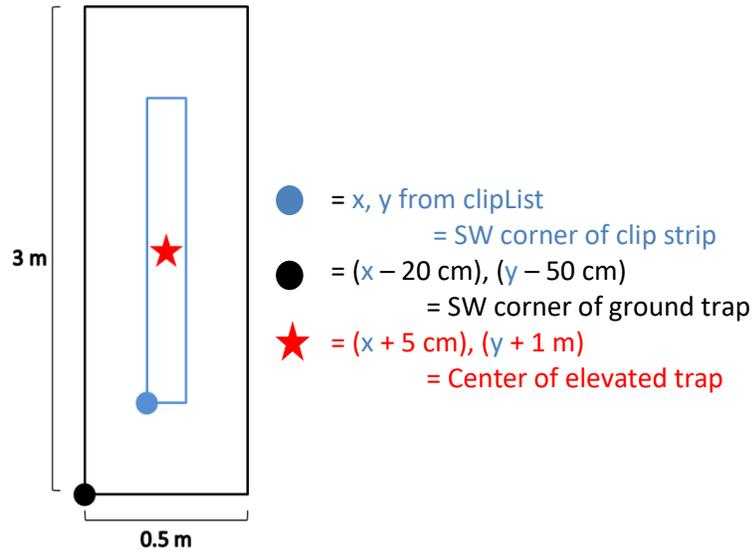
**Figure 2.**  $x, y$ -coordinates for litter trap placement (red star, black circle) differ from coordinates provided in the clipLists provided for use with the herbaceous clip protocol (blue circle) RD[06].
