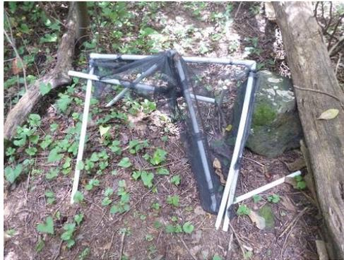
Figure 14. PVC elevated trap destroyed by bears at SCBI.
