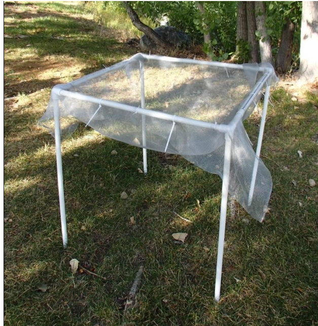
Figure 5. Fully constructed elevated litter trap.
