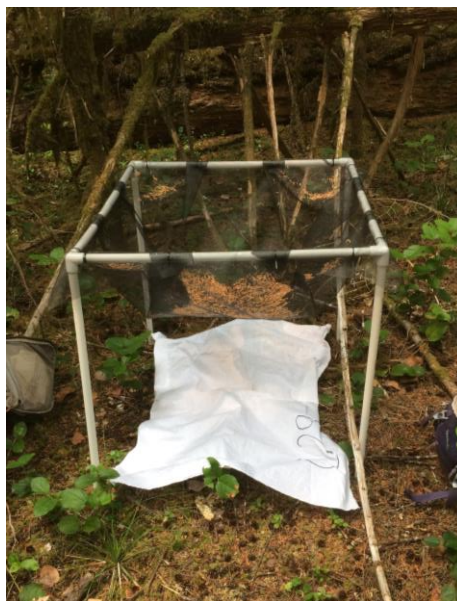
Figure 6. Use of ground cloth to catch trap throughfall.
