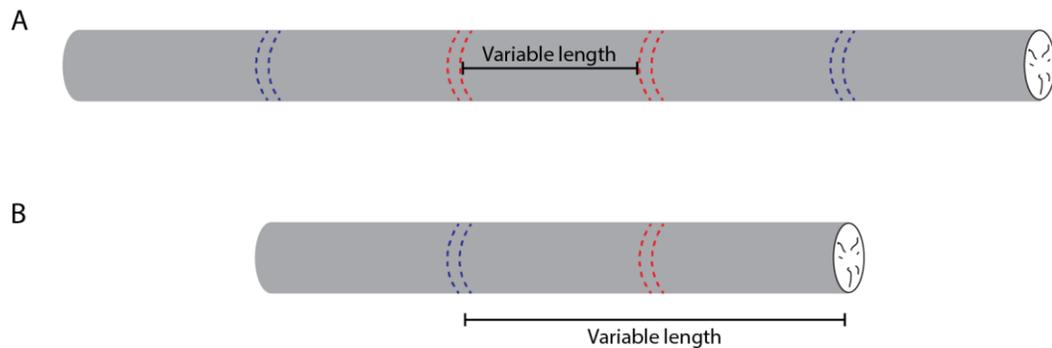
**Figure 6.** Strategy for generating cross-sectional disks from logs re-sampled for bulk density in Bout 2. (A) Logs  $\geq 5$  m length in Bout 1 and  $\geq 3$  m length in Bout 2; (B) Logs  $< 5$  m length in Bout 1 and  $< 3$  m length in Bout 2. Pairs of blue dashed lines represent Bout 1 disks, and pairs of red dashed lines indicate Bout 2 disks.
