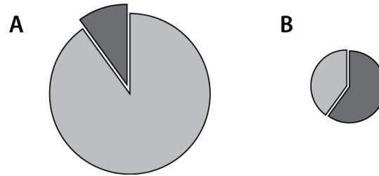
**Figure 5.** Creating wedge-shaped subsamples from cross-sectional disks from relatively large disks (A), and relatively small disks (B). In both A and B, the dark grey area is approx. 100 g, and the light grey is discarded.
