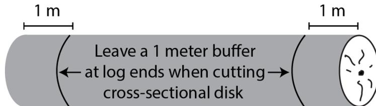
**Figure 3.** A minimum 1 m buffer should be left on either end of a ≥ 10 cm diameter CDW piece when cutting a cross-sectional disk for bulk-density sampling. The log depicted is > 5m length and is sampled from both ends at each of the two sampling timepoints. Qualifying logs < 5m length are only sampled at one end.
