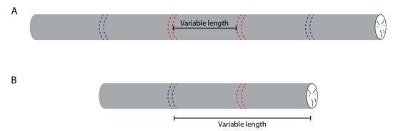
Figure 6. Strategy for generating cross-sectional disks from logs re-sampled for bulk density in Bout 2. (A) Logs  $\geq$  5 m length in Bout 1 and  $\leq$  3 m length in Bout 2; (B) Logs  $\leq$  5 m length in Bout 1 and  $\leq$  3 m length in Bout 2. Pairs of blue dashed lines represent Bout 1 disks, and pairs of red dashed lines indicate Bout 2 disks.
