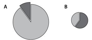
**Figure 5.** Creating wedge-shaped subsamples from cross-sectional disks from relatively large disks (A), and relatively small disks (B). In both A and B, the dark grey area is approx. 100 g, and the light grey is discarded.
