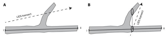
**Figure 3**. A log with a simple fork may be skipped (A) or tallied (B) depending on where the LIDS transect intersects the central axis. (A) The transect misses the central axis, defined as the line between i and ii, and the log is not tallied. (B) The transect intersects the central axis and diameter measurements for the log and fork are made perpendicular to the central axis; the  $RD_E$  of the log + fork are used to determine whether the log is tallied.
