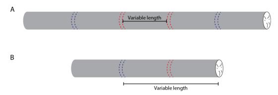
**Figure 8**. Strategy for generating cross-sectional disks from logs re-sampled for bulk density in Bout 2. (A) Logs  $\geq$  5 m length in Bout 1 and  $\geq$  3 m length in Bout 2; (B) Logs < 5 m length in Bout 1 and < 3 m length in Bout 2. Pairs of blue dashed lines represent Bout 1 disks, and pairs of red dashed lines indicate Bout 2 disks.
