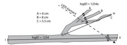
**Figure 4**. LIDS transect intersecting a log with compound forks in two different size categories. Forks in different size categories are assigned unique and related logIDs. The central axis for the main log is defined by the capped line connecting i-ii, and the central axis for the smaller size category compound forked branch is defined by the iii-iv capped line. Measurement locations for each are marked with ellipses.
