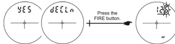
**Figure 2.** The TruPulse viewfinder, showing a user-entered declination value.
