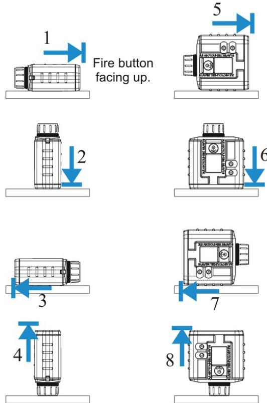
**Figure 6.** The TruPulse tilt-sensor calibration routine.
