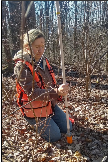
Figure 11. A reflective surface mounted to a staff and held at ground level for using the TruPulse 360R in Target Mode = Filter (Flt). Note the person holding the staff has her eyes closed to avoid looking directly at the laser.
