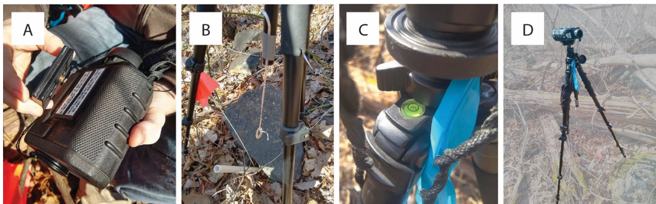
Figure 8. Mounting the TruPulse 360R to a non-magnetic tripod for acquiring high-precision horizontal distance measurements. (A) Attaching the tripod mounting plate to the TruPulse 360R; (B) centering the mounted unit and tripod over a measurement point with a plumb-bob; (C) leveling the unit; and (D) the completed setup ready to collect measurements.
