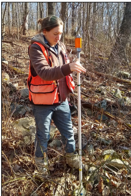
Figure 9. A reflective surface mounted to a staff and held at breast height for using the TruPulse 360R in Target Mode = Filter (Flt). Note the person holding the staff has her eyes closed to avoid looking directly at the laser.
