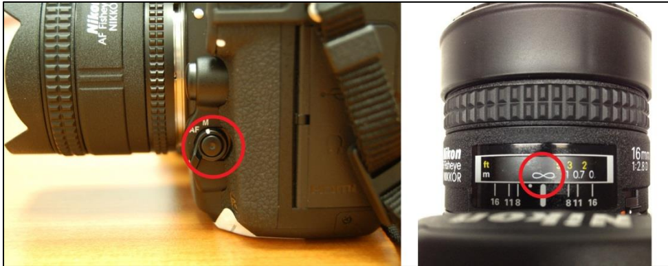
Figure 26. Nikon D750: Focus mode switch, with auto-focus selector button in middle of switch.
