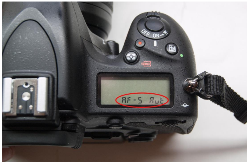
Figure 26. Nikon D750: Top LCD display when camera is configured for single-servo auto-focus auto-mode, where the camera software automatically determines which of the 51 available focus points are used to focus the lens on the subject.
