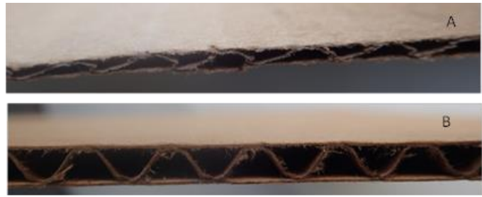
Figure 3. Ventilators with crushed corrugations and fully expanded corrugations. Ventilators with crushed corrugations (image A) should not be used to press and dry specimens because they cannot channel air to dry the plant. Instead, use ventilators with fully expanded corrugations (image B). Ventilators with crushed corrugations (image A) are ideally suited for use during mounted specimen glue drying and as family separators in the herbarium cabinet.
