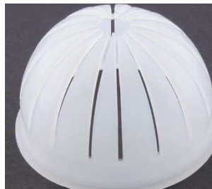
Figure 1 Example soil core catcher that comes with the AMS Multi-Stage Sampler
