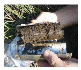
**Figure 2**. Example of a typical wetland soil core demonstrating a poorly defined boundary between O and M horizons (Photo credit: US Environmental Protection Agency). Note that gloves should be worn by NEON technicians when handling soil samples.
