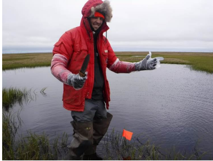
Figure 5 Technician preparing to collect an O horizon monolith in Alaska, using shoulder-length gloves and a hori hori.
