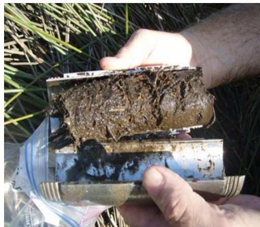
Figure 6. Example of a typical wetland soil core demonstrating a poorly defined boundary between O and M horizons (Photo credit: US Environmental Protection Agency). Note that gloves should be worn by NEON technicians when handling soil samples.
