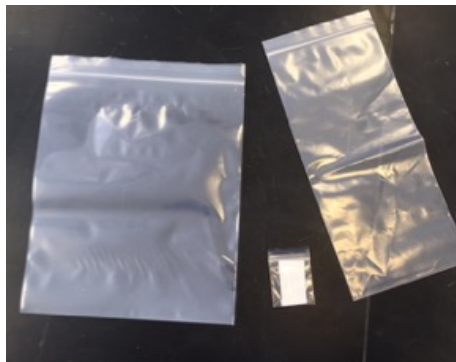
Figure 2 Different size bags to use for N-transformation incubations. Small bag is for the sample ID.
