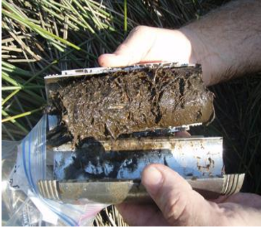
Figure 7. Example of a typical wetland soil core demonstrating a poorly defined boundary between O and M horizons (Photo credit: US Environmental Protection Agency). Note that gloves should be worn by NEON technicians when handling soil samples.
