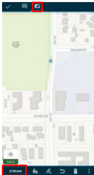
Figure 14. The Stream icon is used to collect a polyline in Arc Collector app.
