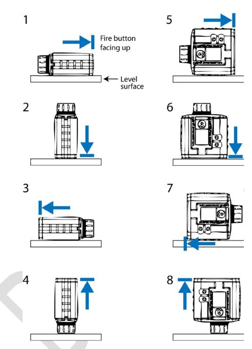
Figure 4. The tilt-sensor calibration routine for the TruPulse 360R instrument. The blue arrow and line indicate the direction of the lens at each calibration step.
