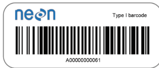
Figure 6. An example of a Type I barcode. These large-size, field-tolerant barcodes have a prefix of 'A' followed by 11 numbers.
