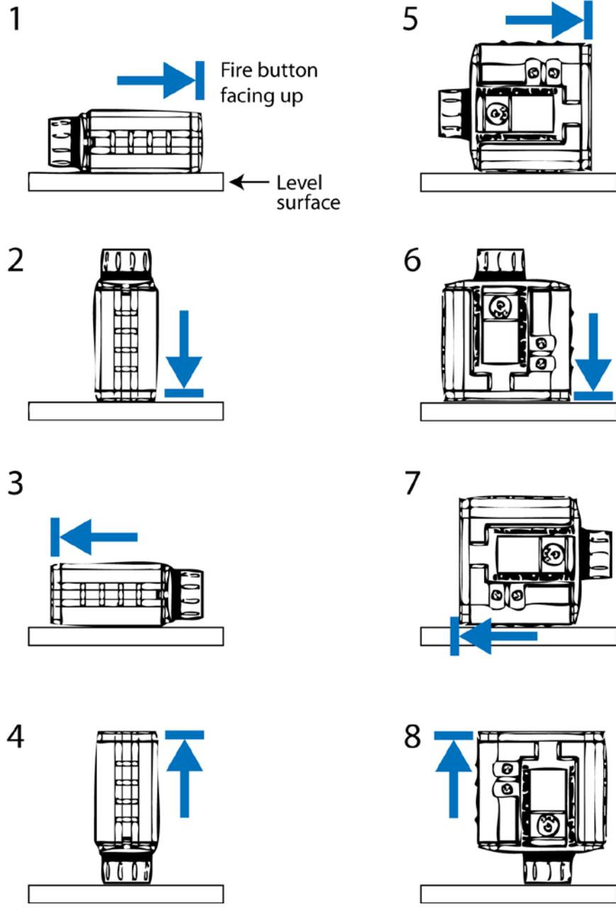
**Figure 7.** The tilt-sensor calibration routine for the TruPulse 360R laser rangefinder. The blue arrow and line indicate the direction of the lens at each calibration step.
