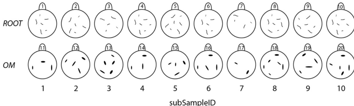
**Figure 6.** Pairs of labeled aluminum weighing tins for separating roots from OM in residual fraction sub-samples. Mixed sub-samples are initially transferred to the *OM* tins, and roots are then sorted into the *ROOT* tins.
