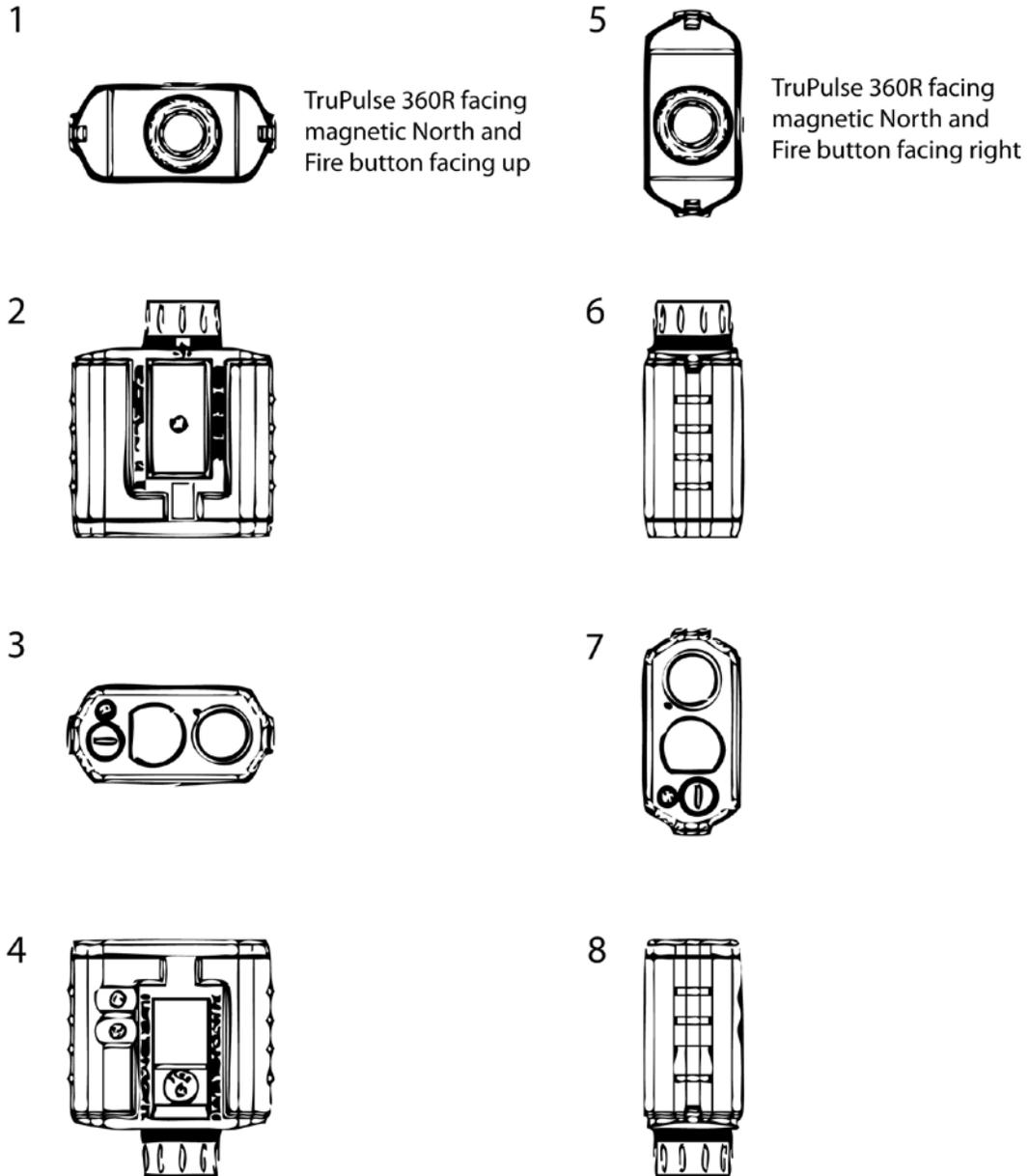
**Figure 8.** The internal compass calibration routine for the TruPulse 360R laser rangefinder.
