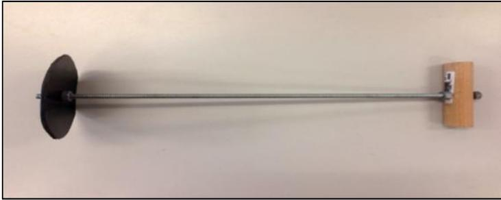
**Figure 3.** Assembled plunger used to randomize root fragment samples < 1 cm length as part of dilution sampling (SOP D).
